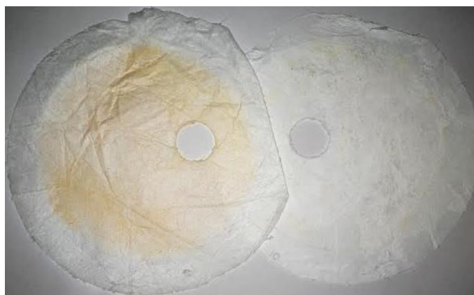
Figure 3-15. Fabrics after the fluorescein aerosol testing; left = "blank", right = 1 wt/v% BTA.
