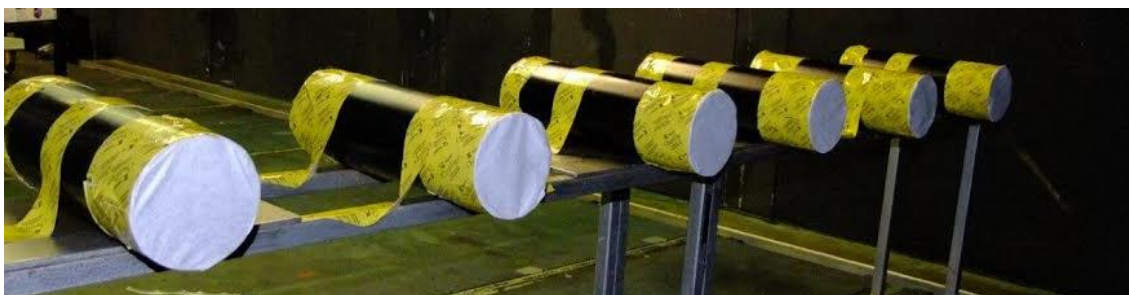
Figure 2-52. Demonstration of the 6 samples run each test within the wind tunnel; 3 blanks and 3 treated.
