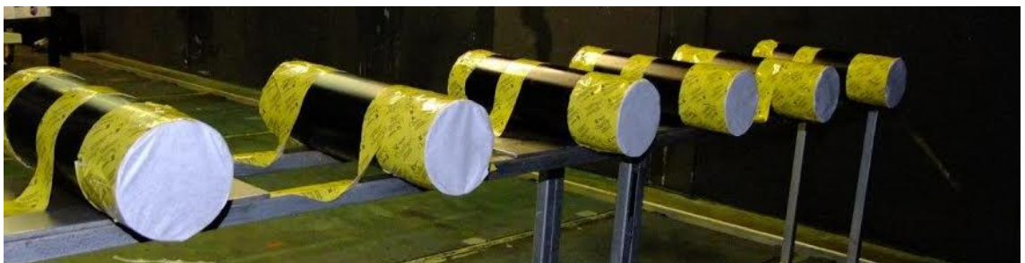
Figure 8-3. Demonstration of the 6 samples run each test within the wind tunnel; 3 blanks and 3 treated.
