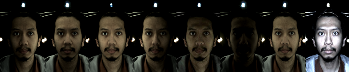
Figure 4.11: The eight images captured in a sequence. Starting from the leftmost, the X , Y , Z , \hat{X} , \hat{Y} , \hat{Z} and C are the LED spherical gradient images. The rightmost image is the flash image.
