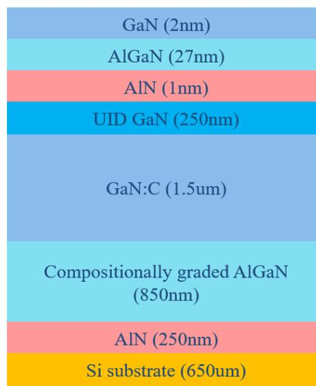
**Figure 2-1 Typical layer structure for all-GaN integrated cascode device.**
