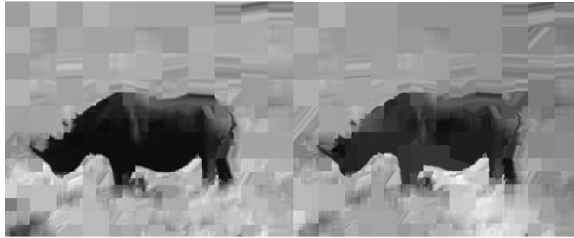
Figure 3-19 : Comparison between original reconstructed prediction data and simplified reconstructed prediction data. Left: original reconstructed prediction frame. Right: simplified reconstructed prediction frame.
