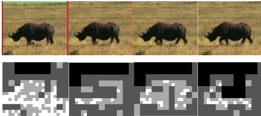
Figure 3-8 Block depth feature map in low delay configuration. First row: original frames in low delay mode. Second row: block depth map in low delay mode.
