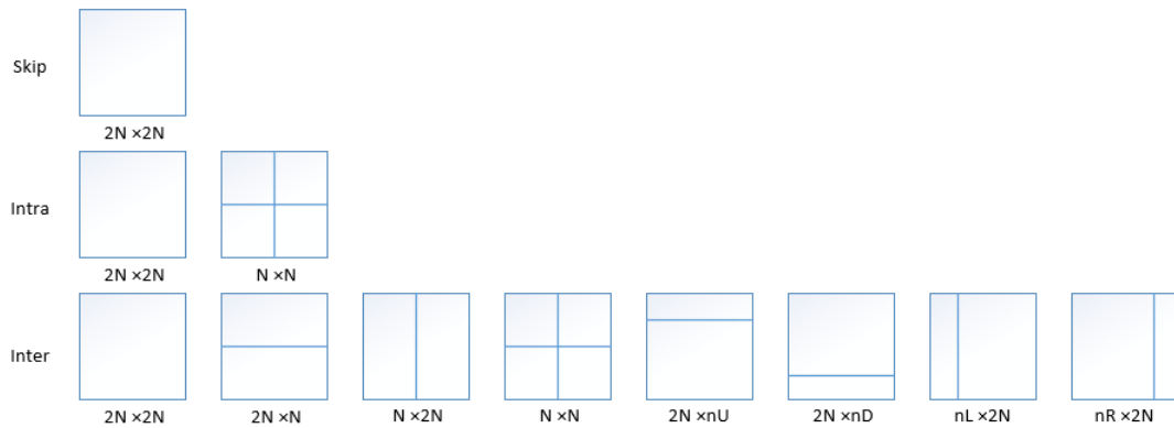
Figure 2-13 The block partitions in HEVC.
