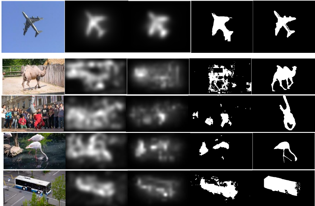
Figure 3-22 Intra-frame saliency results of objects moving with dynamic background set. First column : Original frame. Second column: GBVS image saliency. Third column: Itti's image saliency. Fourth column: Proposed method (Bayesian model). Fifth column: Manual segmented ground truth.
