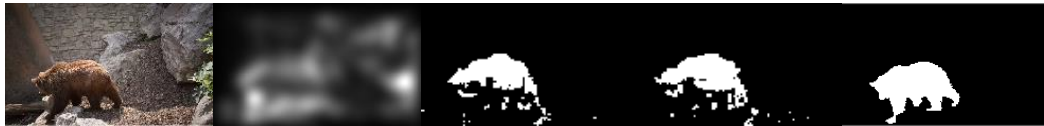
Figure 3-25 Inter-frame saliency results. First column: Original frame. Second column: Itti motion saliency. Third column: Proposed method with low delay configuration. Fourth column: Proposed method with random access configuration. Fifth column: Manually segmented ground truth from dataset.
