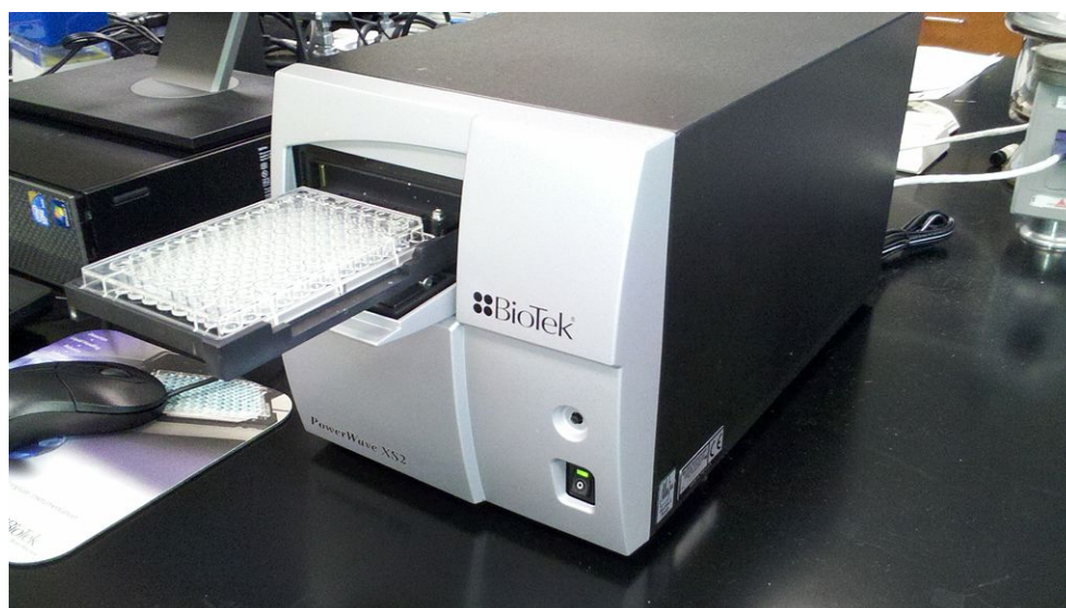
Figure 3.25: Photograph of a typical microplate reader (175). It is essentially a UV-vis spectrophotometer, containing a laser that probe cells at various wavelengths, measuring the absorption or excited emission of the sample, typically to detect for photolabels, similar to the flow cytometer discussed in Section 3.3.2.
