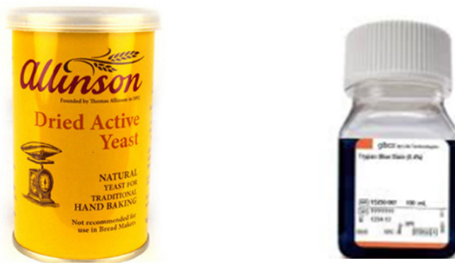
Figure 3.19: Bakers yeast used in these experiments (left), and Trypan blue (right), which selectively stains dead yeast.
