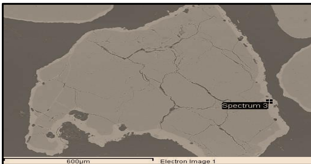
Figure 9-10 EDX Spot Analysis of the mixture of Willow + Wood sample @ 802.0 C (spectrum 3)
