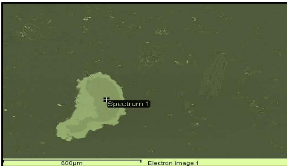
Figure 9-33 EDX Spot analysis of willow sample at 750 °C (spectrum 1)
