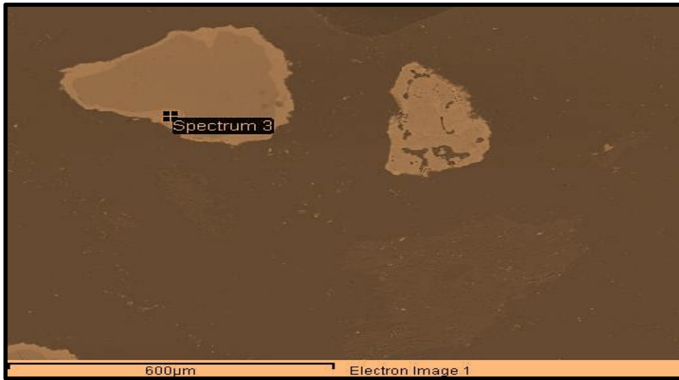
Figure 9-24 EDX Spot analysis of Wood sample @ 750 °C (spectrum 3)
