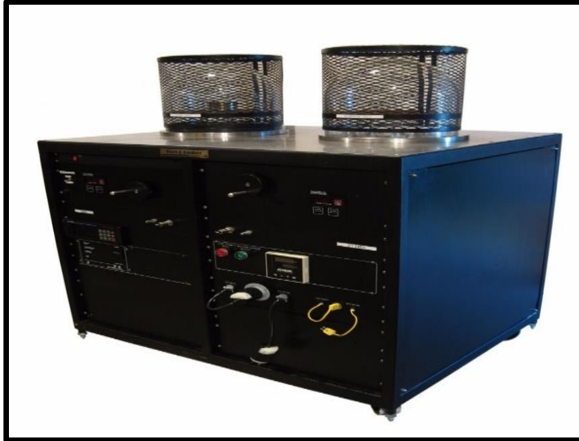
Figure 4-16: Carbon Coating Instrument, Speedivac Coating Unit.
