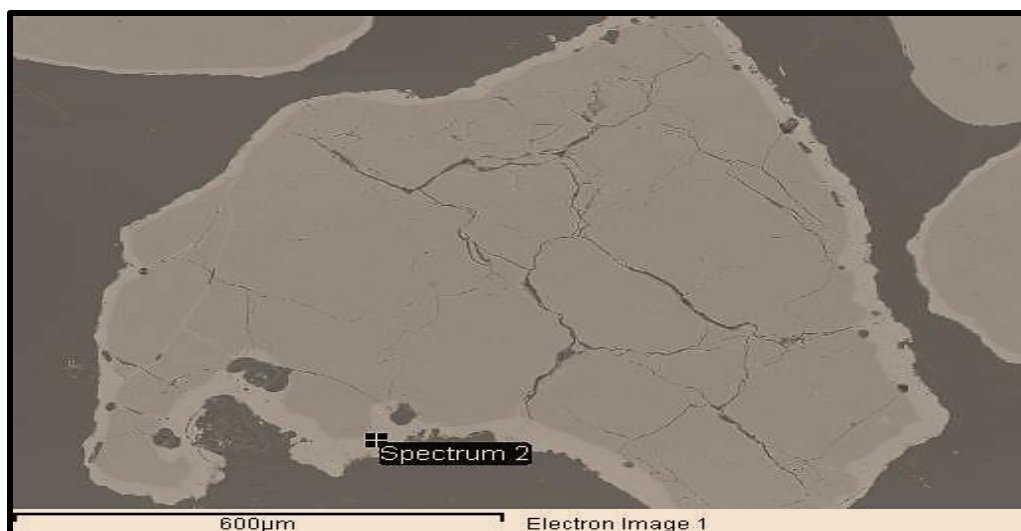
Figure 9-9 EDX Spot Analysis of the mixture of Willow + Wood sample @ 802.0 C (spectrum 2)
