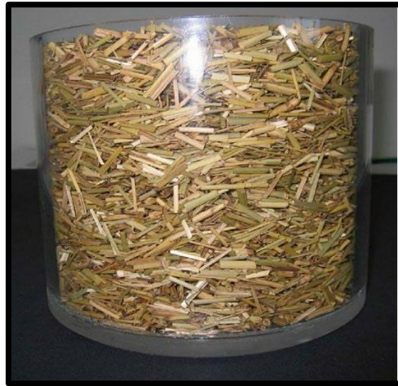
Figure 4-6: Bulk density of mixed particles of switch grass and wheat straw (wet and dry) [228, 231-233]
