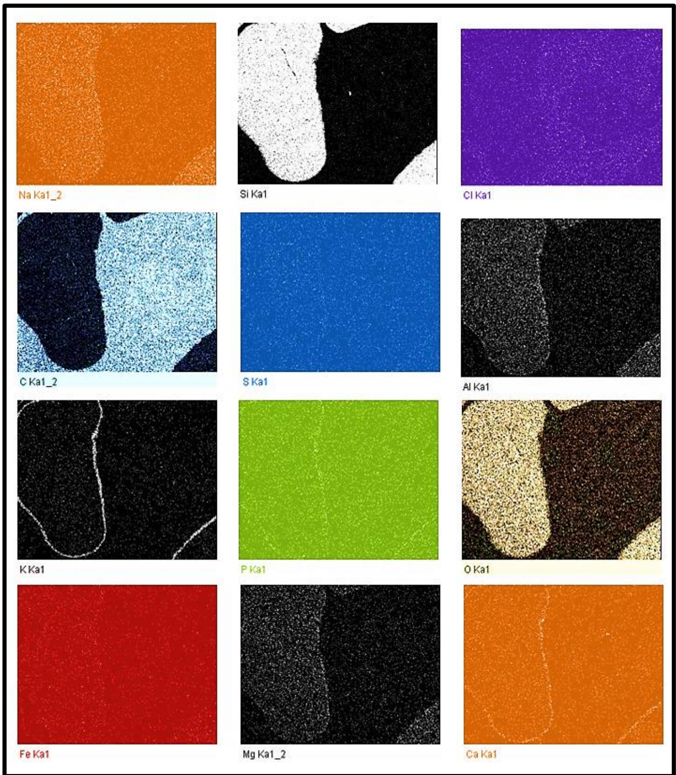
Figure 6-43: Element mapping of panel a in Figure 6.42, mixture of white wood with miscanthus melted at 802 °C.
