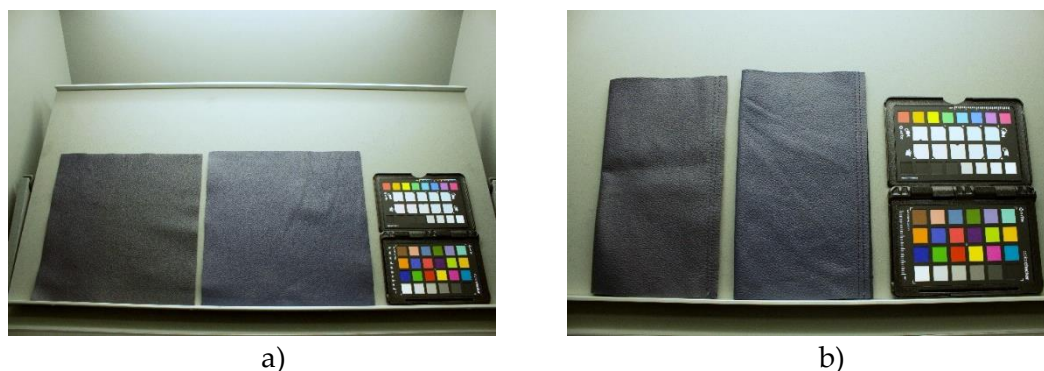
Figure 5-1: Samples of TL cut for visual (a) and crumple-flex (b) before (right) and after (left) Sahara test.
