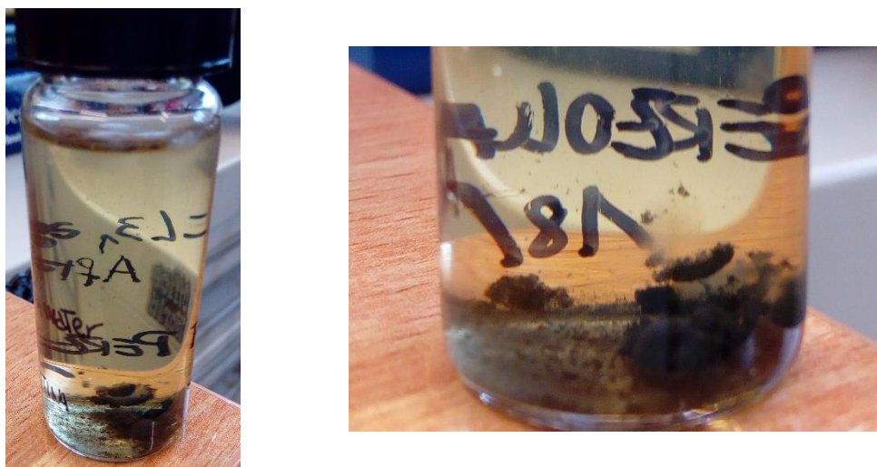
Figure 5-70: Formation of semi-spherical agglomerates after EL3 stirring
