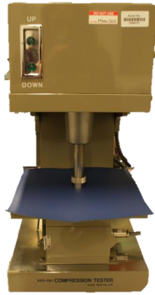
Figure 3-8: Sample during compression test
