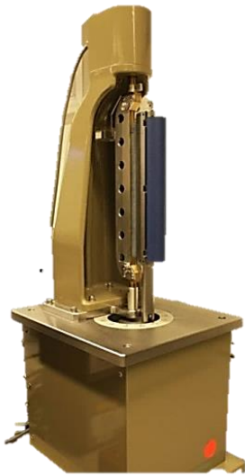
Figure 3-6: Sample during bending test
