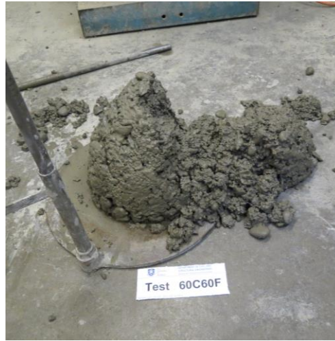
Figure C.58 Collapse of slump test for mix 60CR60FR
