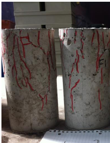
Figure G.22 Failure of mix E1
