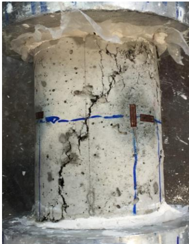
Figure G.53 Failure of 60CR60FR
