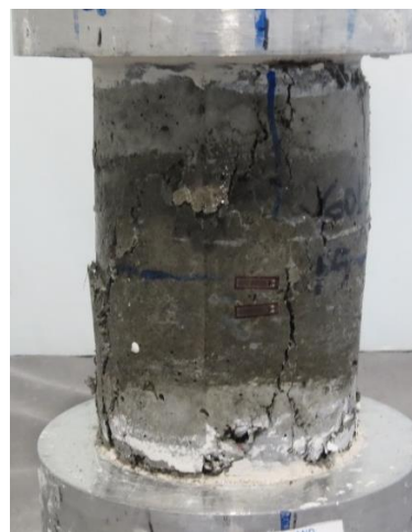
Figure G.57 Failure of 60CR60FR
