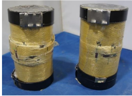
Figure 8. Typical failure modes of AFRP CRuC cylinders
