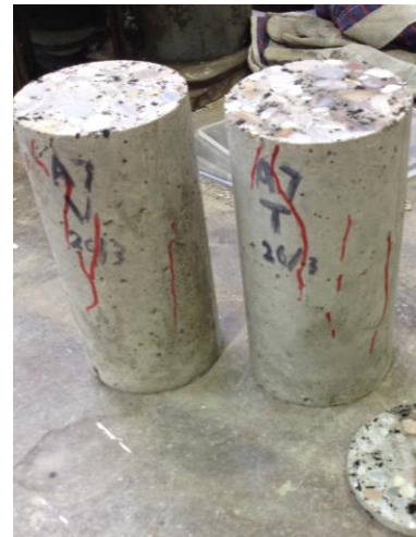
Figure G.14 Failure of mix A5
