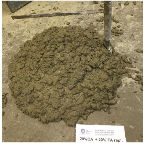
Figure C.53 Slump test for mix 20CR20FR
