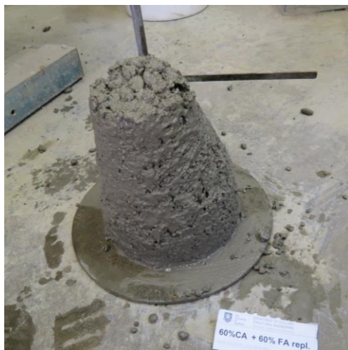
Figure C.57 Slump test for mix 60CR60FR
