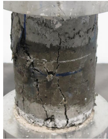
Figure G.52 Failure of 60CR60FR
