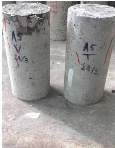
Figure G.13 Failure of mix A5
