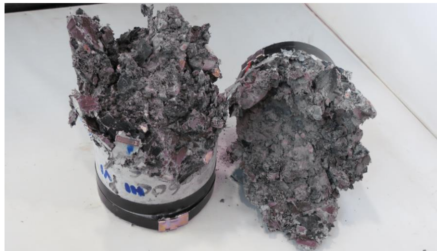
Figure G.49 Broken specimen – 60CR60FR
