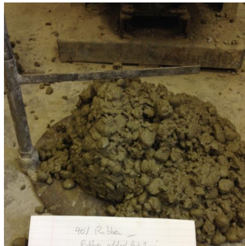
Figure C.35 Slump test for mix E1
