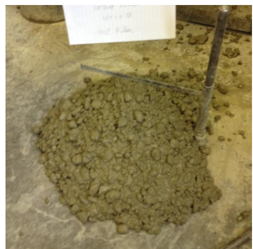
Figure C.10 Slump test for mix A4
