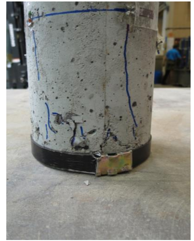
Figure G.35 Failure of 20 CR
