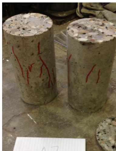
Figure G.15 Failure of mix A7
