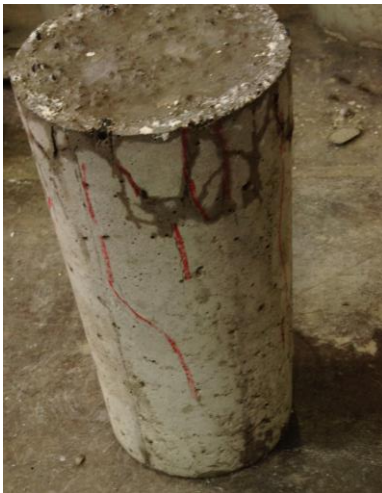
Figure G.12 Failure of mix A1
