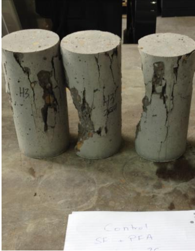
Figure G.24 Failure of plain mix
