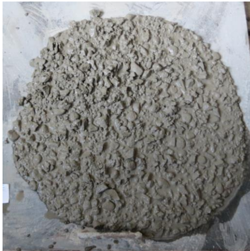
Figure C.48 Flow table test for mix 60CR
