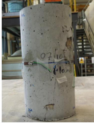
Figure G.25 Failure of plain mix
