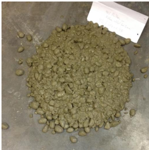
Figure C.34 Flow table test for mix E1
