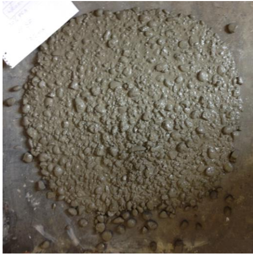
Figure C.32 Flow table test for mix D3
