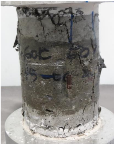
Figure G.50 Failure of 60CR60FR
