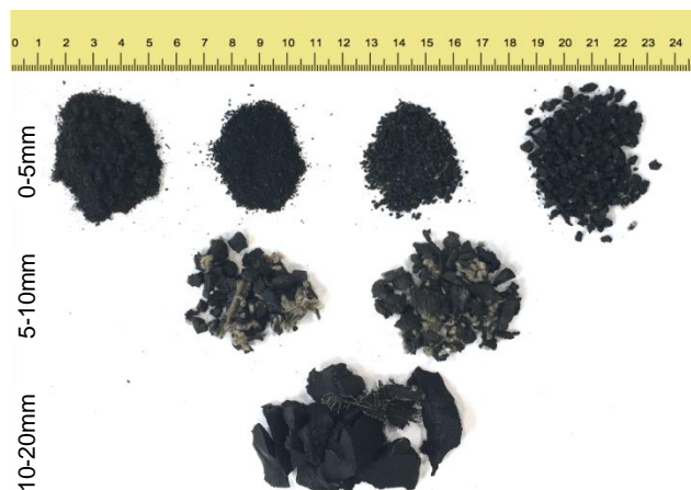
Figure 1. Rubber particles used to replace sand (0-5mm) and gravel (5-10mm and 10-20mm)
