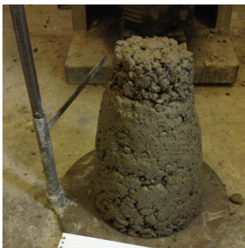
Figure C.14 Slump test for mix A7
