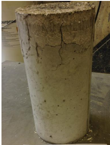
Figure G.5 Failure of mix O3
