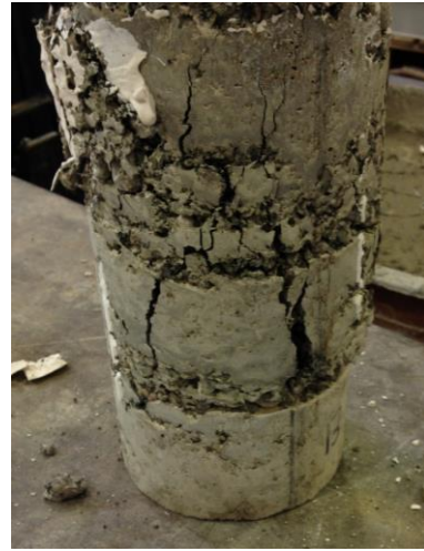
Figure G.11 Failure of mix O2
