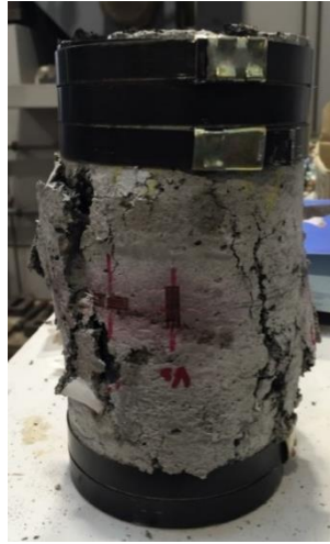
Figure 5. Typical failure of 60F&C RuC cylinders
