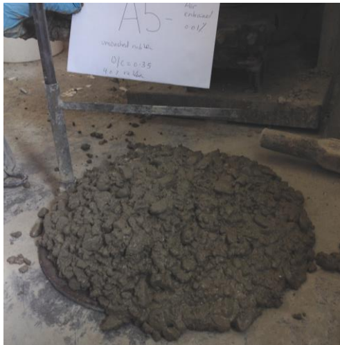
Figure C.11 Slump test for mix A5
