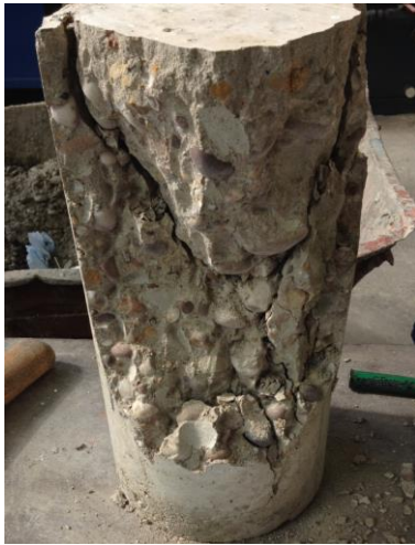
Figure G.1 Failure of mix O1
