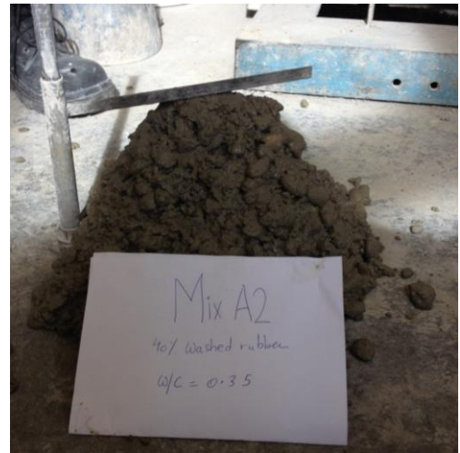
Figure C.6 Slump test for mix A2
