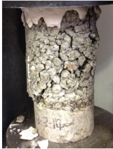
Figure G.10 Failure of mix O4
