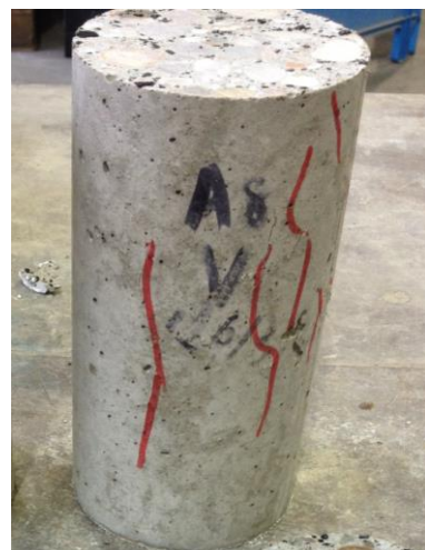
Figure G.17 Failure of mix A8
