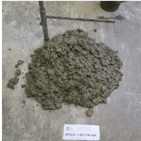
Figure C.55 Slump test for mix 40CR40FR
