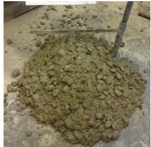
Figure C.8 Slump test for mix A3
