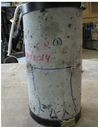
Figure G.36 Failure of 20CR
