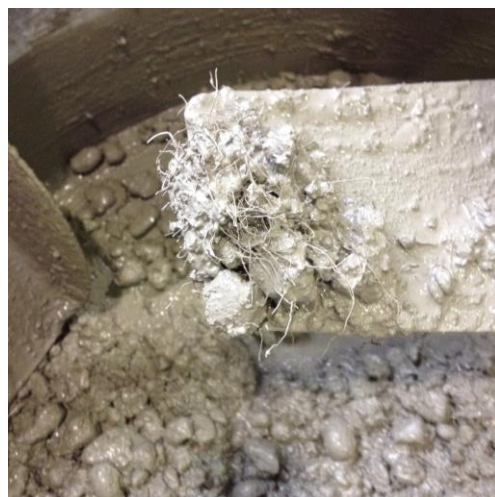
Figure C.36 Appearance of fibre balling in mix I1
