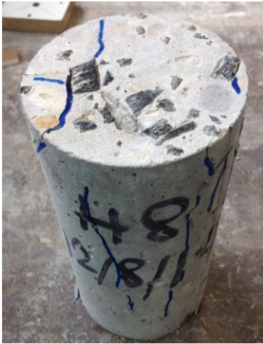
Figure G.39 Failure of 40 CR
