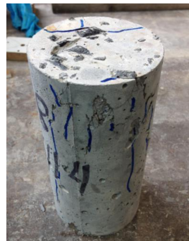
Figure G.37 Failure of 40 CR
