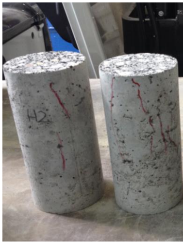
Figure G.28 Failure of 80FR
