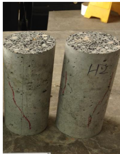
Figure G.29 Failure of 80FR
