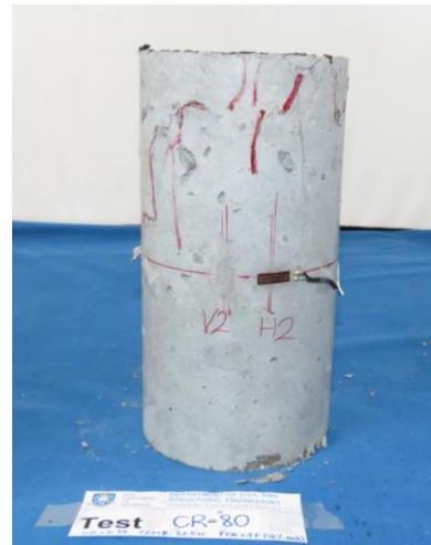
Figure G.44 Failure of 80 CR
