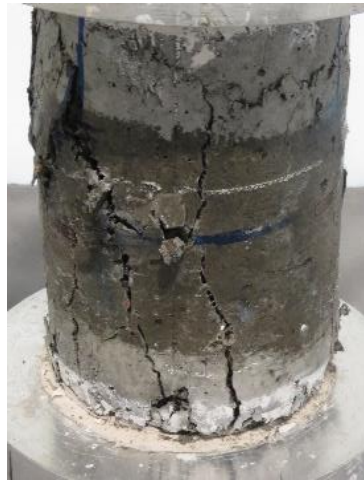
Figure G.51 Failure of 60CR60FR
