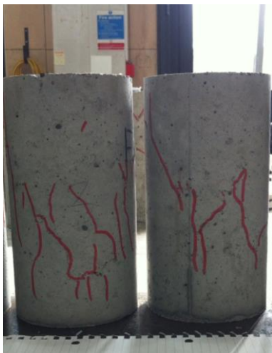
Figure G.21 Failure of mix D2
