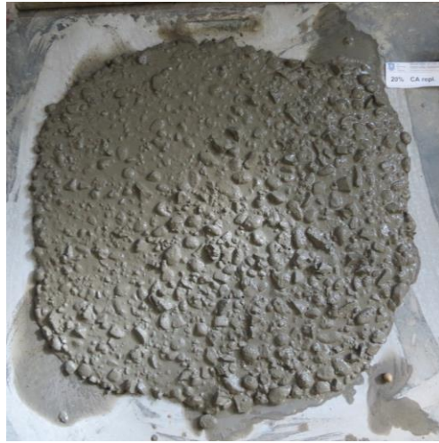
Figure C.47 Flow table test for mix 20CR
