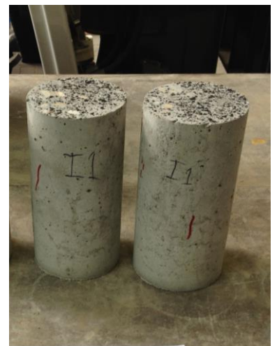
Figure G.23 Failure of mix I1
