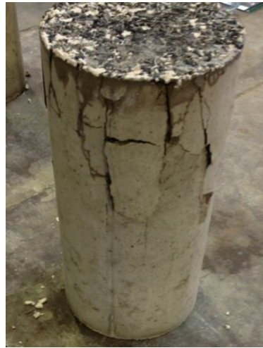
Figure G.2 Failure of mix O2
