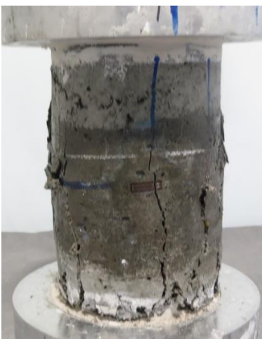
Figure G.56 Failure of 60CR60FR
