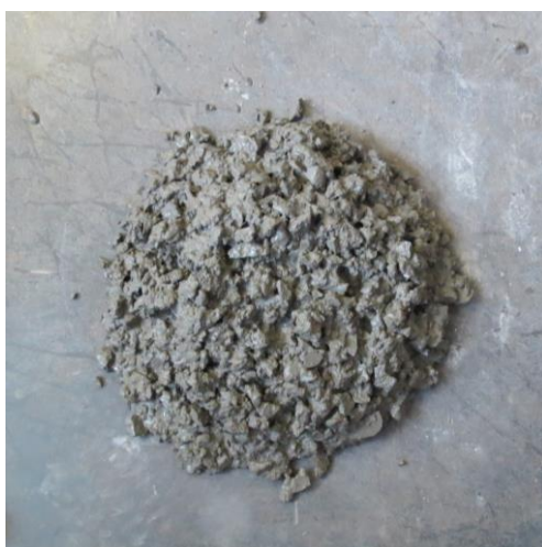
Figure C.50 Flow table test for mix 100CR
