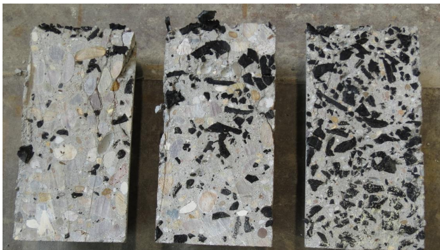
Figure G.45 Section view of 20CR (left), 40CR (middle) and 100 CR (right)
