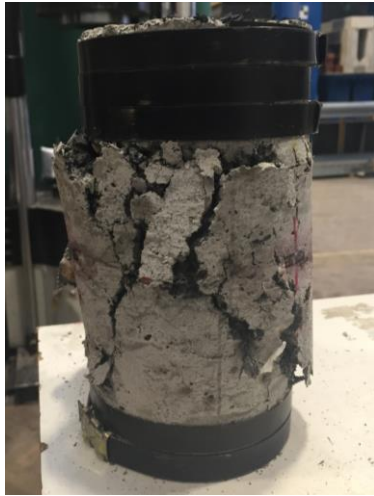
Figure G.46 Failure of 60CR60FR
