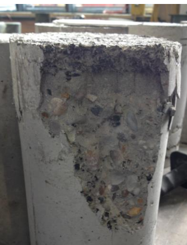
Figure G.7 Failure of mix O3
