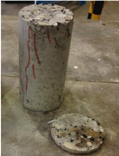
Figure G.18 Failure of mix D1
