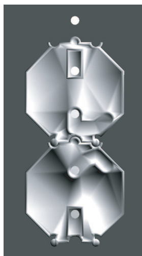
FIGURE A.1: Miyashita-type design where paths for folding are asymmetric. The distance between magnets in paths decreases monotonically but there is difficulty during experiments in moving a magnet along the path that is not angled.
