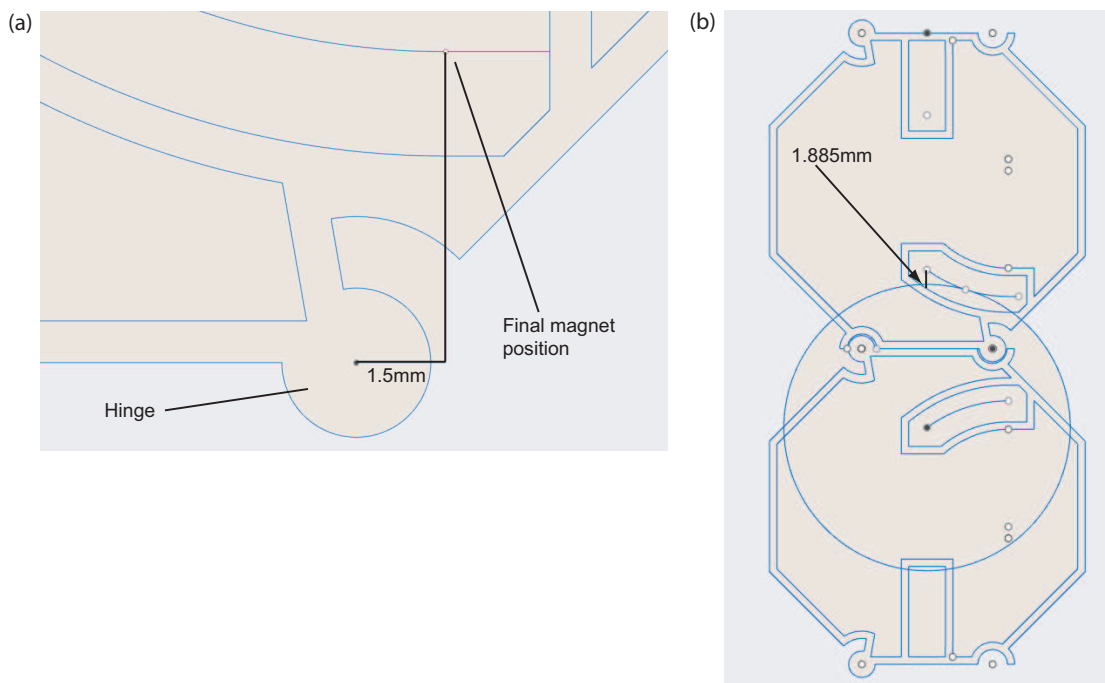
FIGURE 6.4: Considerations during the design of curved paths. (a) Location of final positions for magnets in curved paths. (b) Overhead view of two tiles with curved paths. Circle is centred at the initial position of the third magnet in the chain, showing the point on the path of the second magnet where they will be closest in distance. The third magnet must be able to begin moving before the second magnet reaches this point in order for propagation to be possible.
