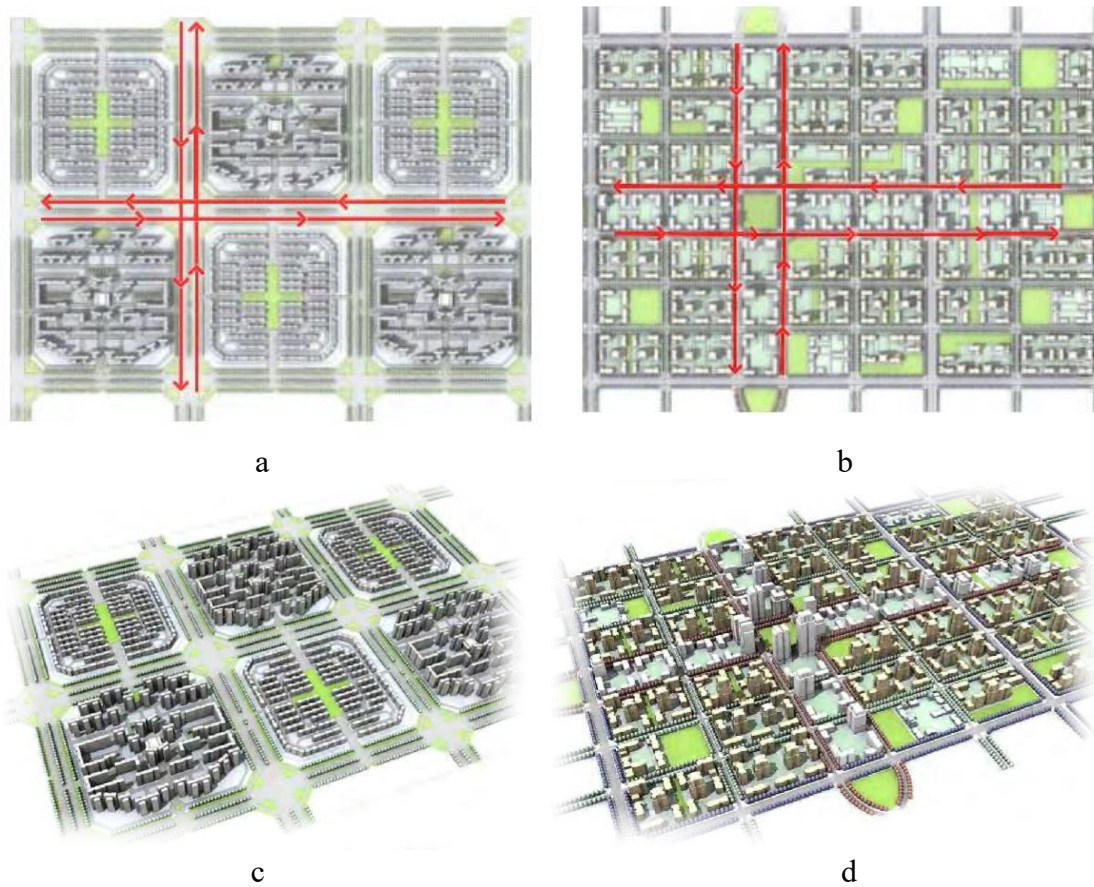
Figure 2.14 Illustrations of typical building massing within a Superblock System and an Urban Network: (a) and (b), Super block plan; (c) and (d), small block plan. Source: Calthorpe Associates (2012).
