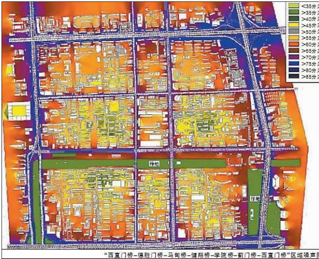
Figure 2.19 The first official noise map of China, a 12.7 Km 2 pilot noise-mapping project combining multiple methods, including in-situ measurement, EU noise mapping technique and GSI. Source: Beijing Daily (Cai, 2009)
