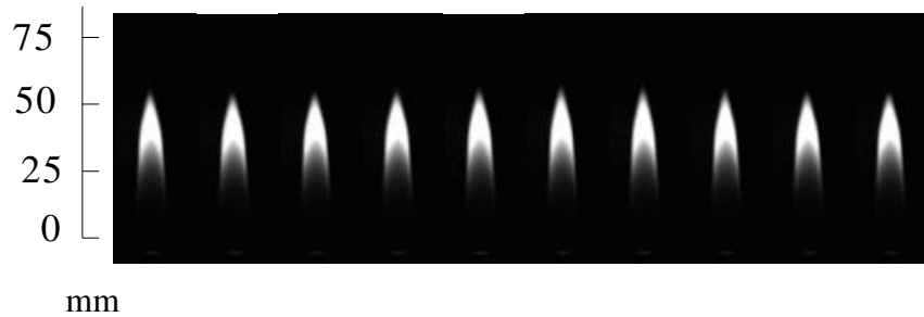
(a) Direct imaging sequence with the fuel flow rate at 0.3 l/min and co-flow air flow rate at 7 l/min (The time interval between each two images is 10 ms)
