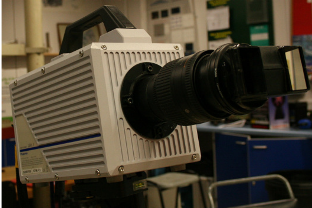
Figure 3-2 High speed camera with Pentax stereo adapter attached in front of the lens
