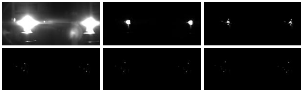
Figure 6-9 Stereo images of the ignition spark without air flow jet (The time interval between each two images is 1 ms.)
