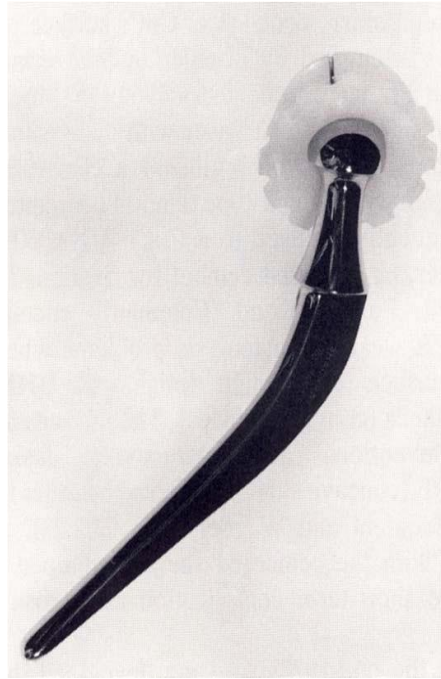
Figure 1.5 Hard-on-soft THR bearings, The Charnley Total Hip Replacement (Buechel and Pappas, 2012)
