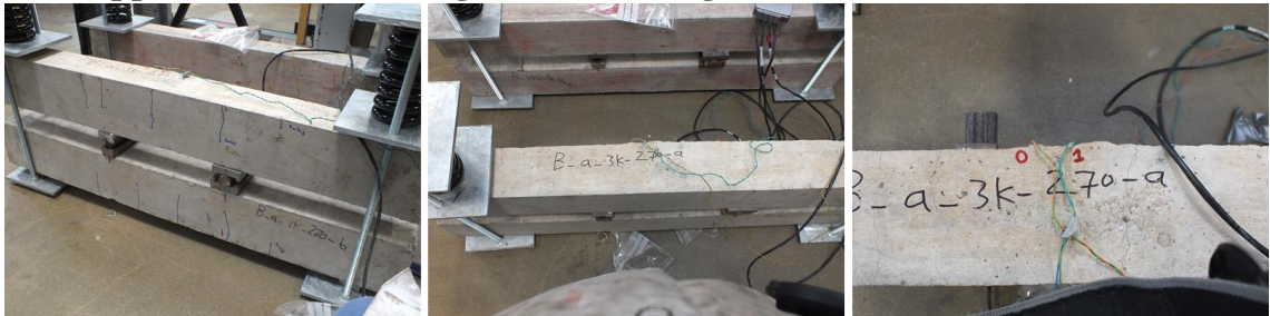
Figure.III.2 sustained load application
