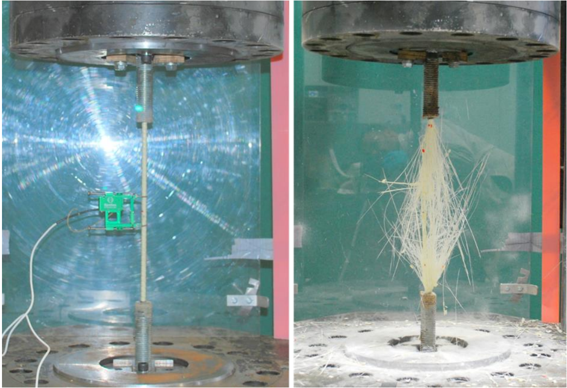
Figure 3.9: Details of the tensile test set-up and failure mode
