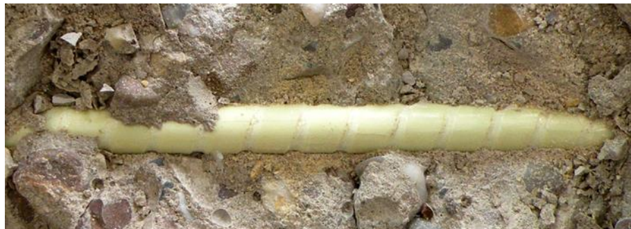
Figure. 5.6: Extracting the bars from conditioned unstressed specimens
