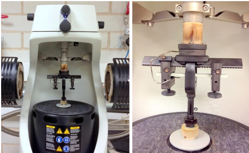
Figure 3. 12: Details of glass transition test using a DMA machine
