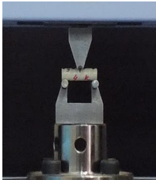
Figure 3. 10: Inter-laminar shear test
