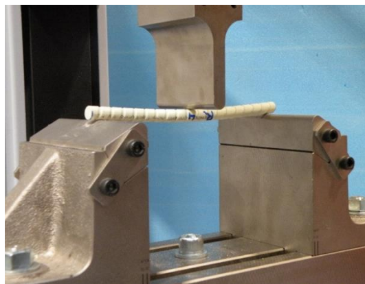
Figure 3. 11: Test set-up for flexural test on FRP bars
