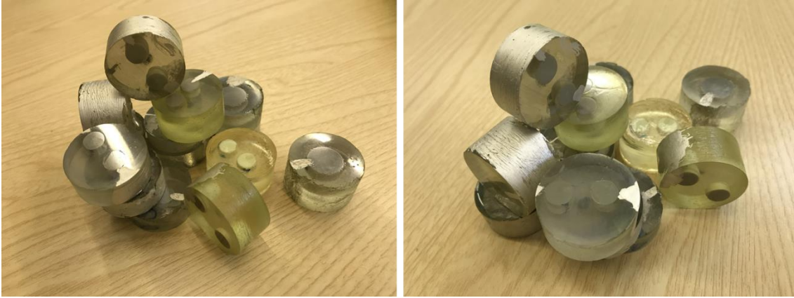
Figure.II.15: SEM specimens at different conditions and time
