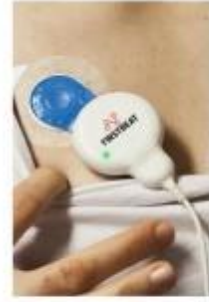
4. The measurement starts automatically when the device is attached. Make sure the green led is flashing. NOTE: The light is easiest to see in a dark room.
