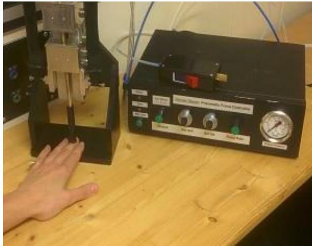
Figure 3.1 The pneumatic pressure pain stimulator used in the studies of this thesis (manufactured by DancerDesign, St. Helens, UK). A series of pressure pain stimuli were applied to the finger tip of the middle finger at three intensities: non-painful, pain threshold, and moderately painful (as set for each participant individually using a ramping procedure).
