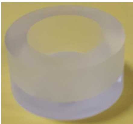
Figure 4.16 Holder cup used for the polished powders mounted in transoptic resin.
