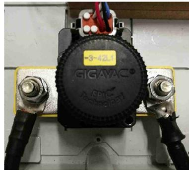
Fig. 6-5 Turn fault emulating relay
