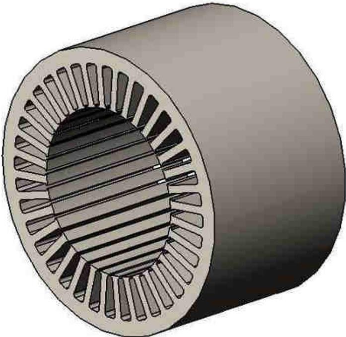
Fig. A-2. Skewed stator stack
