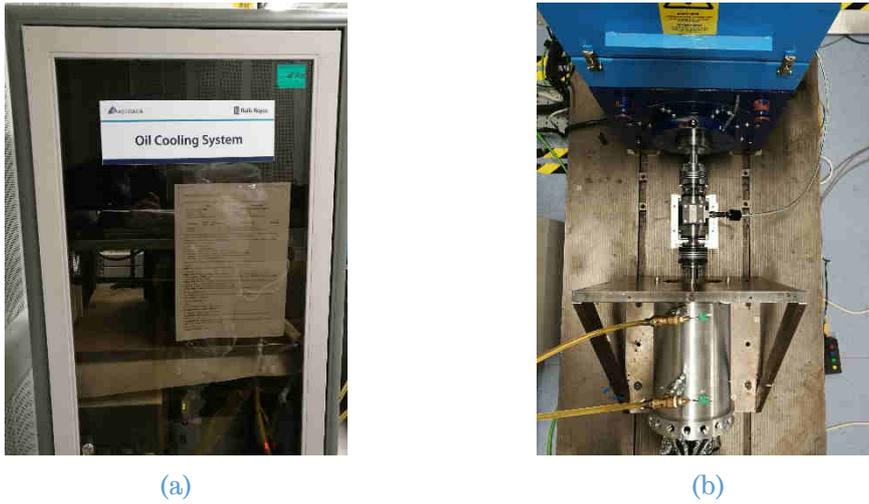
Fig. 6-9 Oil cooling system (a) oil cooling pump (b) cooling pipes and connections
