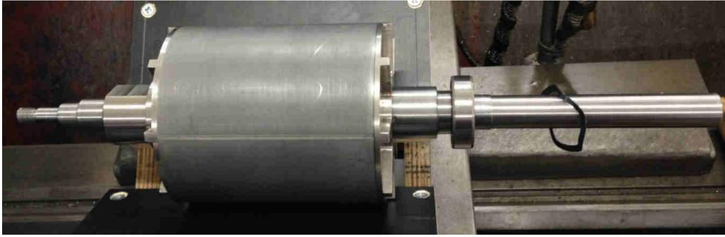
Fig. 6-2 Rotor assembly
