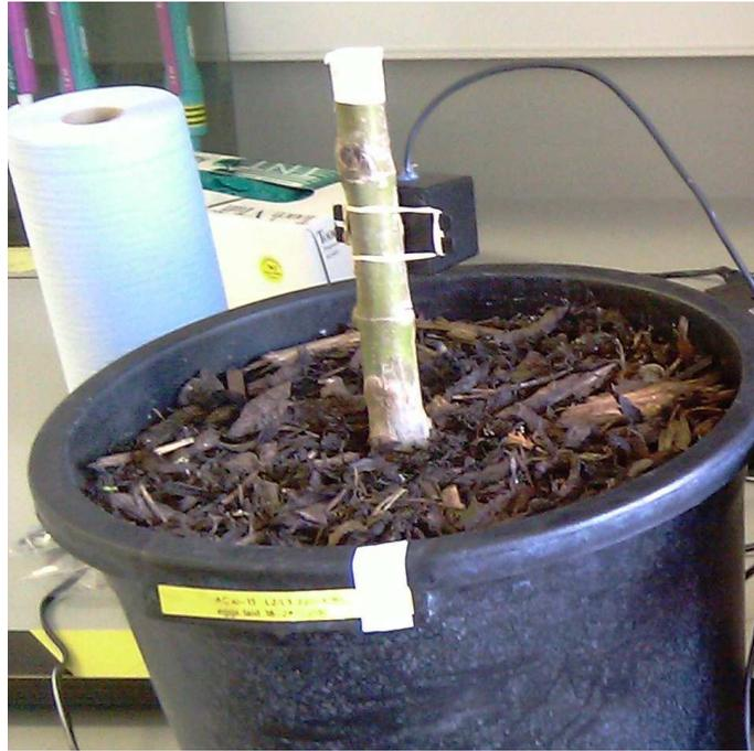
Figure 6.4: Sensor attached using rubber bands
