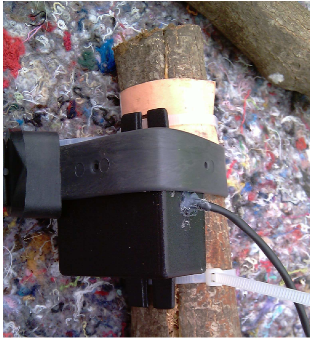
Figure 6.3: Sensor attached using a tree strap
