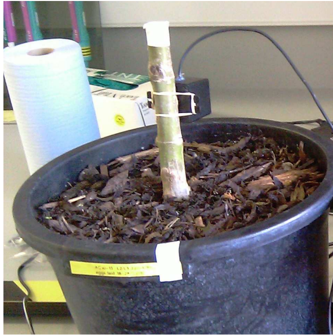
Figure 6.4: Sensor attached using rubber bands
