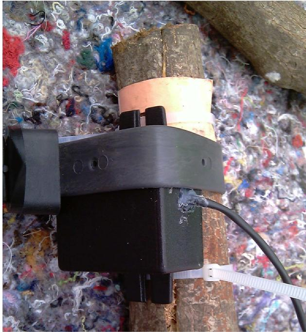
Figure 6.3: Sensor attached using a tree strap
