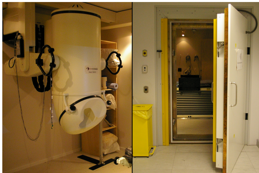
Figure 4.2. An MEG dewar (left) positioned within a magnetically-shielded room (right).
