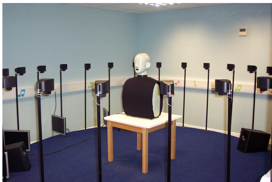
Figure 7.3. The head and torso simulator placed in the centre of the loudspeaker array. The height of its in-ear microphones and the loudspeakers were approximately equal.
