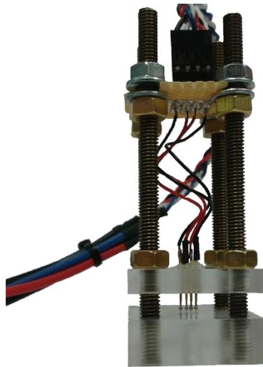
*Figure 4.18. Photograph of the custom built four probe system.*
