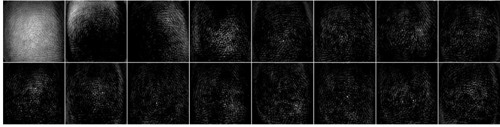
Figure 6.37: 16 out of a total 39 of eigendiffusion faces of fingerprints
