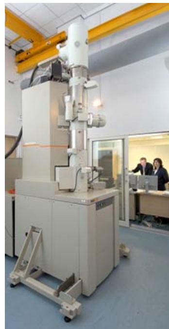
Figure 1.19 a) Diagram of a Transmission Electron Microscope. b) Field Emission Transmission Electron Microscope 37
