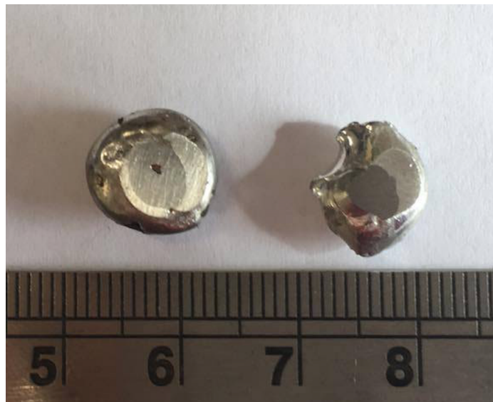
Figure 5.6: The significant macro-segregation that is found in the alloys as part of the silver single phase HEA search. The sample on the left is AgSingle2 and the sample on the right is AgSingle3. Scale shown is in cm.
