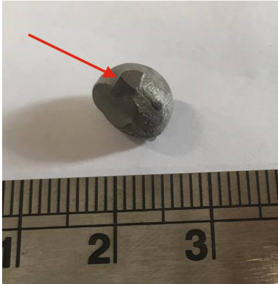
Figure 5.12: A photo of the unsuccessful melt of HOSP-6-5. Shown on top of the sample is the end of an unmelted tantalum rod, shown by the red arrow. Scale shown is in cm.
