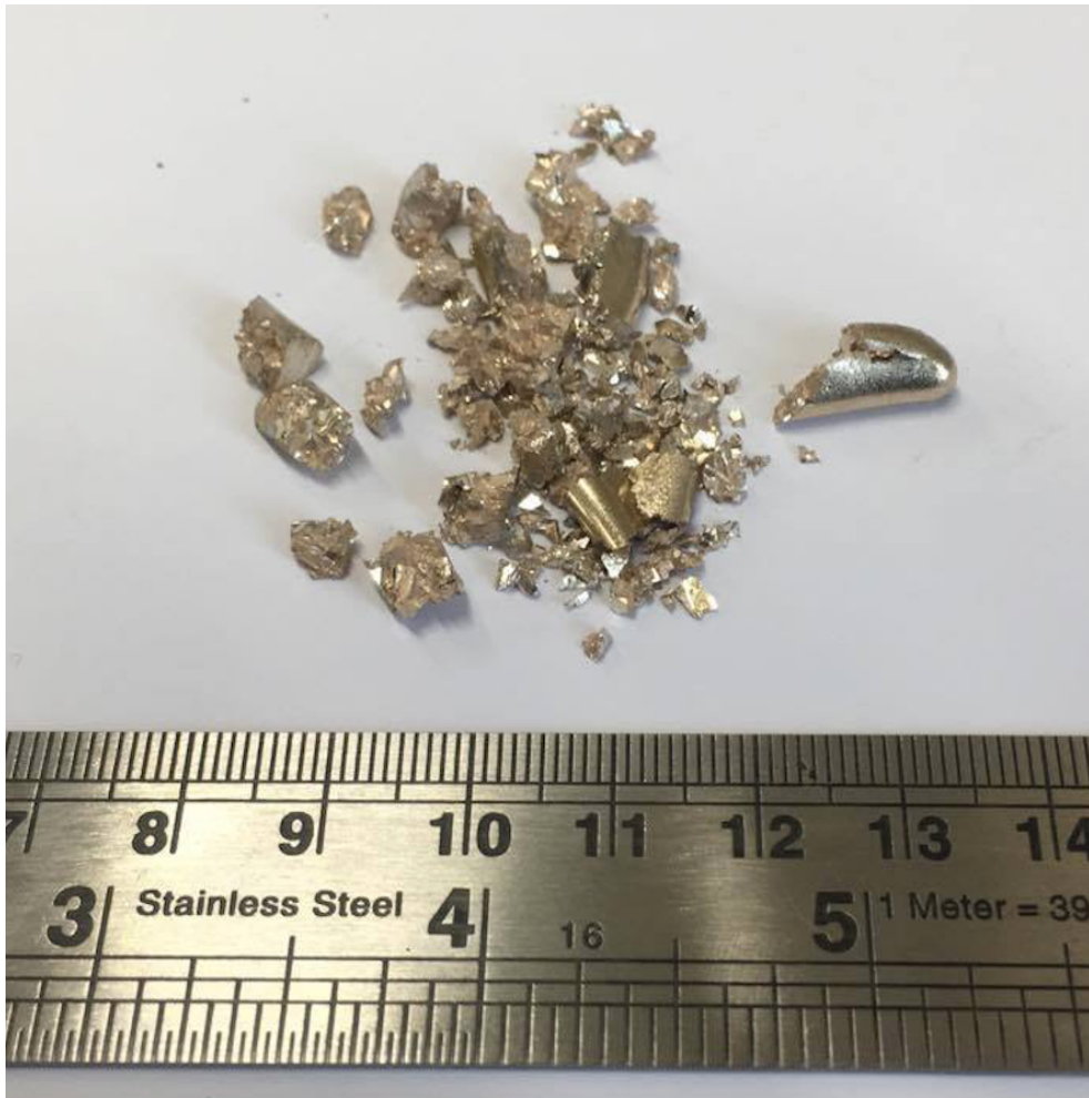
Figure 3.19: NBA11 after one pass of the rolling ductility test. The roll gap was less than 1mm smaller than the thickness of the sample.
