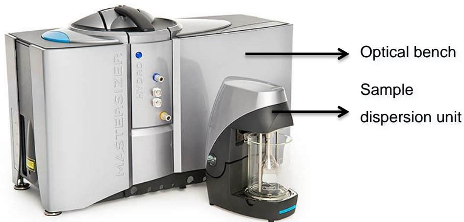
Figure 5.16. Main device used in analysing bed particle sizes (taken from Malvern, 2017).
