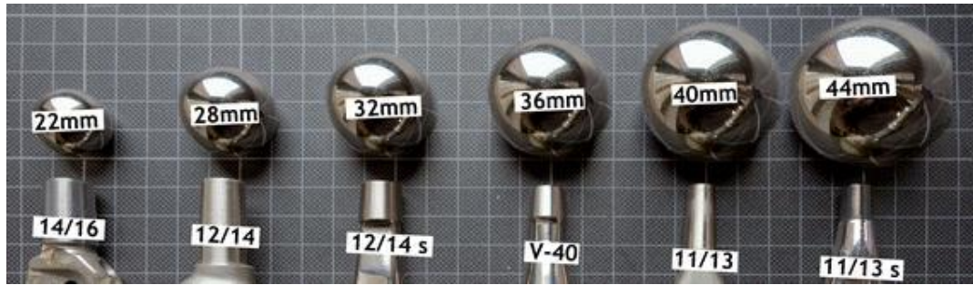
Figure 3-3 – Increasing bearing sizes from left to right and decreasing taper sizes in the same direction [57].
