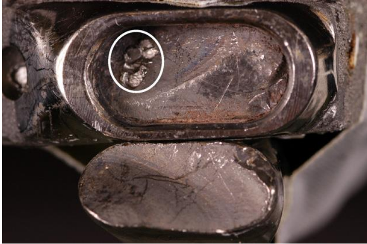
Figure 3-9 – Fracture of the neck component at the neck-stem interface [81]
