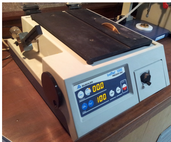
Figure 2.6: Buehler precision saw (model Isomet 1000) from Department of Archaeology at University of York. The saw was used for sectioning the sea shells in this study.
