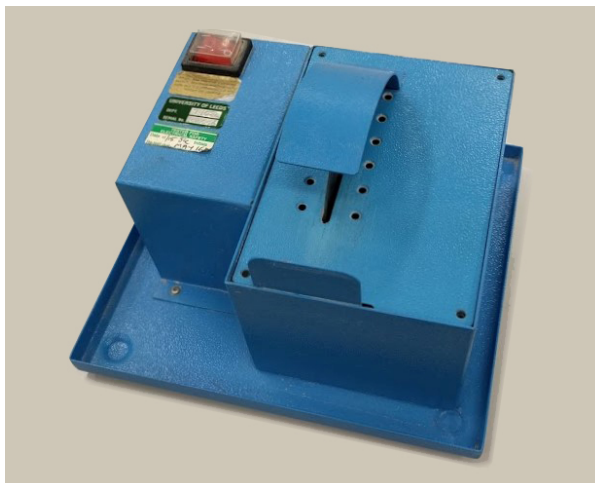
Figure 2.8: ML Beach Faceters Trim Saw from the Thin Section Lab at the University of Leeds.
