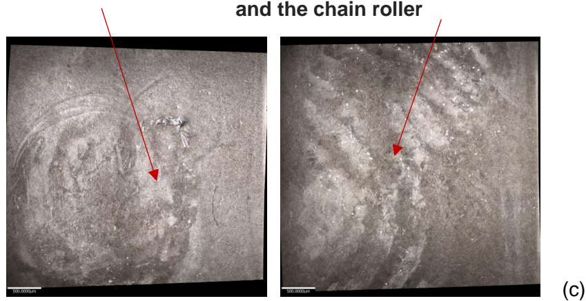
Figure 8.21: 2D surface images of the chain roller specimen (a) pre-test in its true and pseudo colour of the surface with height differences, (b) 0wt%CB content 12-hour test and (c) 0wt%CB content 24-hour test
