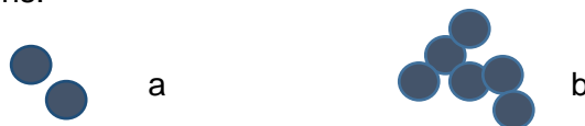
Figure 3.1: The depictions of: (a) Soot as elemental particles and (b) a chain agglomerate of soot particles
