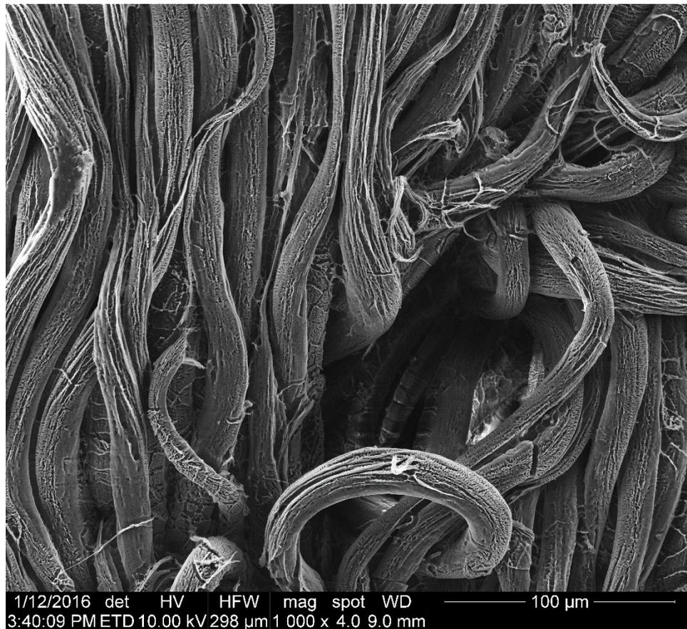
**Figure 5.19 - Pores created in a great amount of fibres in MWov fabrics (FA pre-treated and subsequently ozone treated in UHP for 96 h)**
