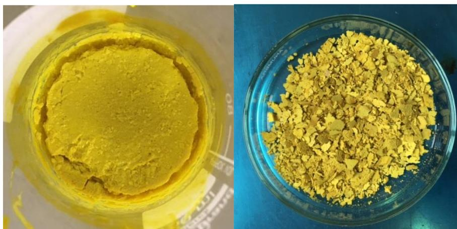
**Figure 3.11 - (a) PIM during precipitation process; (b) PIM crude product**
