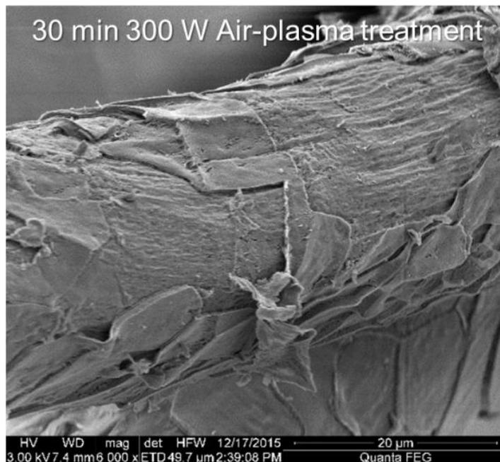
**Figure 5.14 - Air plasma treated FA pre-treated MFH fibres**
