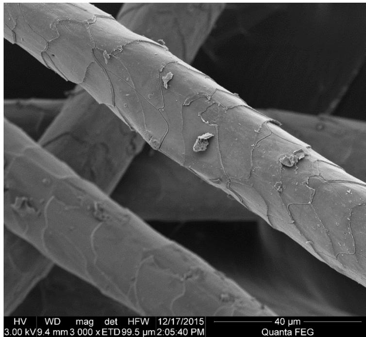
**Figure 5.13 - Air plasma treated raw MFH wool fibres**
