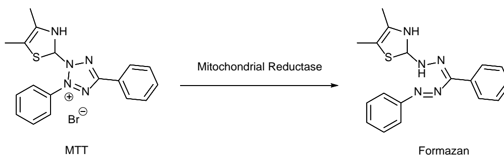
Scheme 1. Reaction scheme of MTT being converted to Formazan. 11
