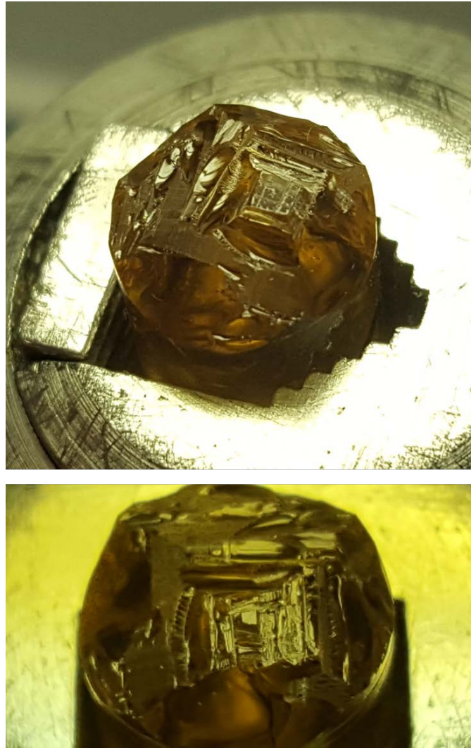
Figure 12. Resin block roughly trimmed to the area of interest with a razor blade (top) and the final trimming and shaping of the resin block ready for sectioning (bottom).
