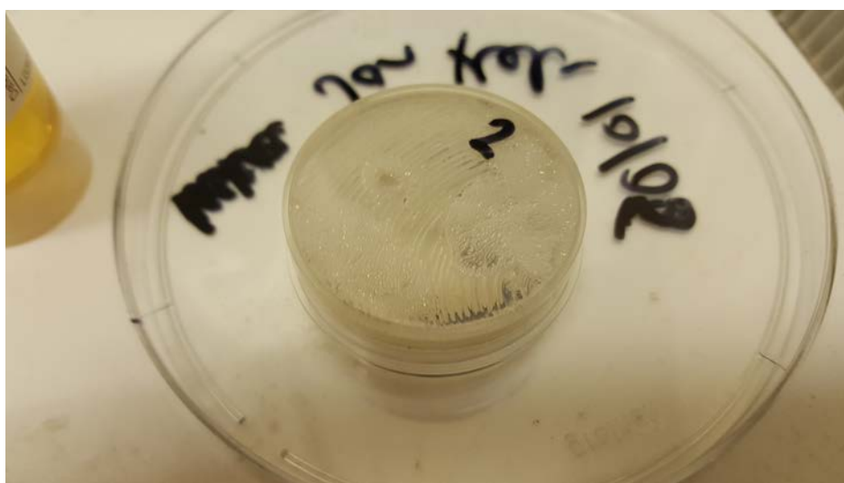
Figure 9. Lid of the Ibidi plate displaying erosion from the intermediate solvent, propylene oxide.
