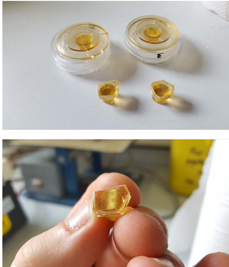
Figure 10. Ibidi 35 mm plates with the resin blocks heat shocked to remove the coverslip with the excess resin visible in the further samples (top) and a close up of the resin block after trimming showing the transferred grid pattern (bottom).
