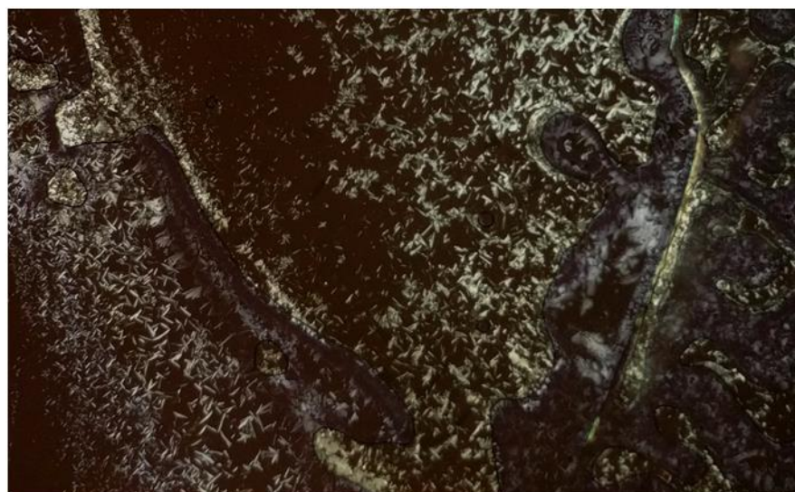
Figure 4.8: Polarising optical microscopy images [Fan-C 12 -SB-C 12 ][BF 4 ] at 69 °C after cooling from the isotropic liquid phase at 10 °C min -1 .
