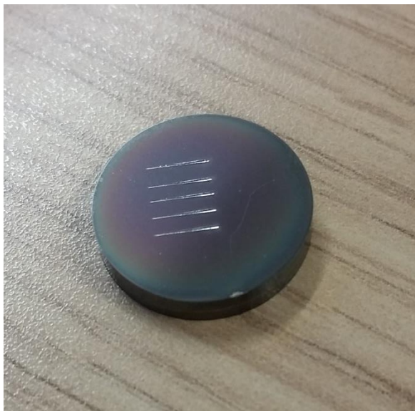
Figure 3.19: A silicon nitride coated coupon following scratch testing; five scratches were made on each coupon, which were subsequently analysed using a light microscope to identify locations of failures associated with critical loads.
