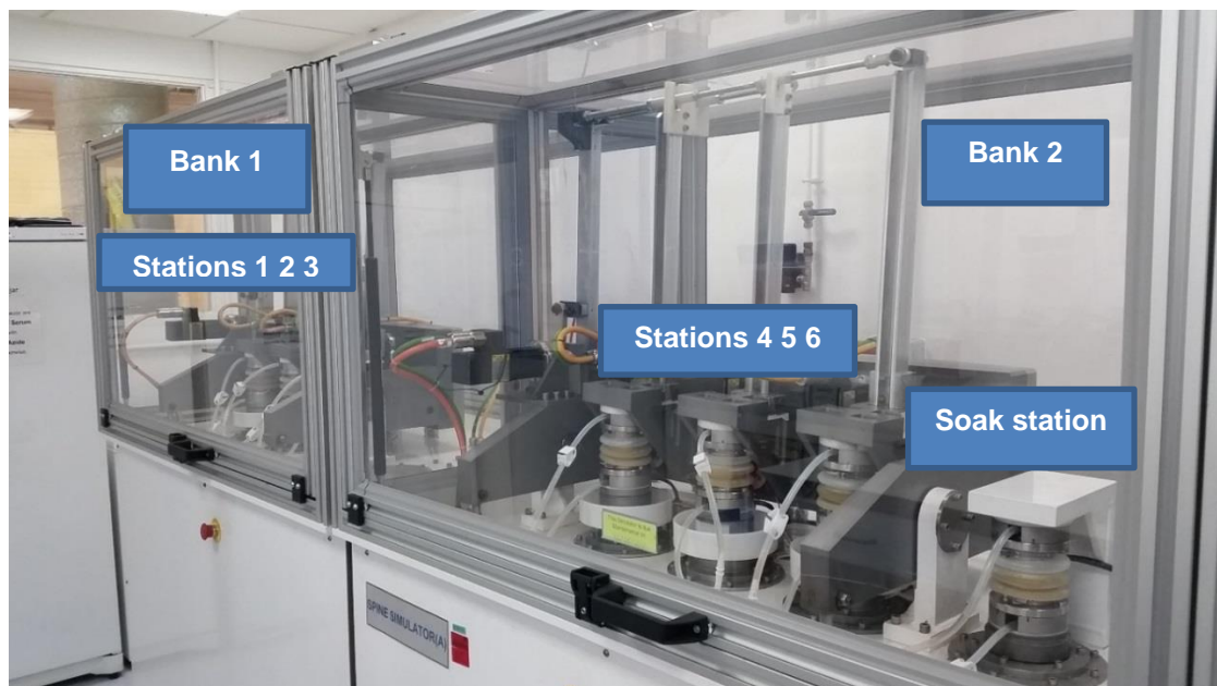
Figure 4.1: Leeds Spine Simulator A showing Banks 1 and 2 with stations 1-6 and a soak station
