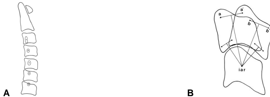
Figure 1.13: A - Mean instantaneous axes of rotation for each motion segment of the cervical spine depicted with a dot. Two standard deviation range of distribution is located within the enclosed circles shown. B - The position of IAR can change position during motion and can be determined by superimposing tracing of a vertebrae in full ROM [28].
