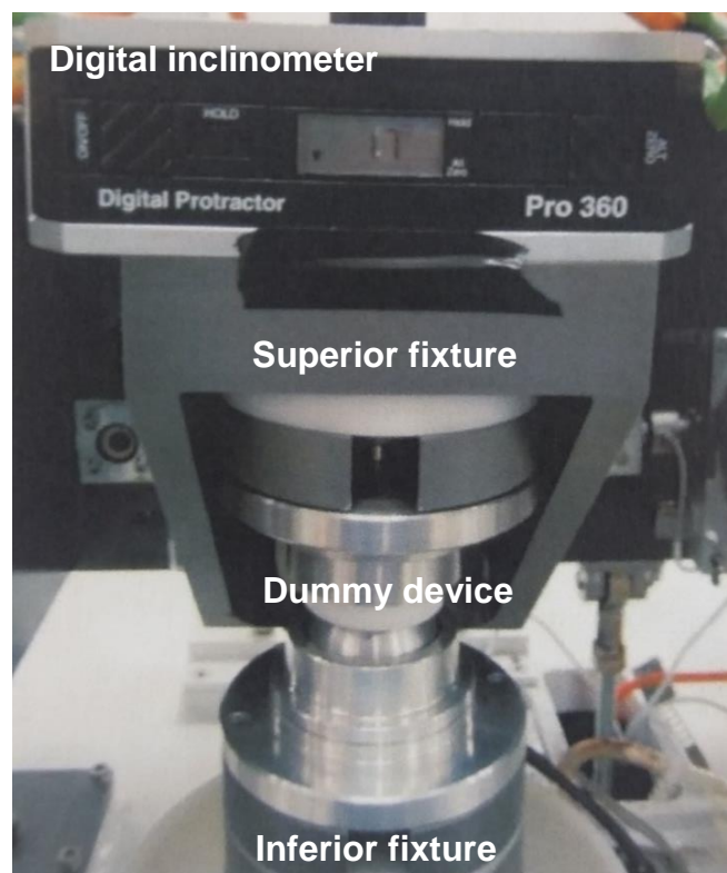
Figure 4.4: Set up for flexion-extension calibration using a digital inclinometer.
