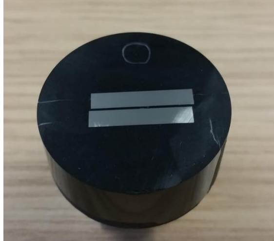
Figure 3.5: Fractured silicon nitride-coated sample embedded in the Bakelite resin.
