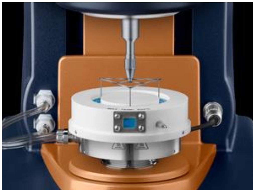
Figure 4.6 Image of a stress-controlled Discovery Hybrid Rheometer equipped with a double wall ring (DWR) geometry.
