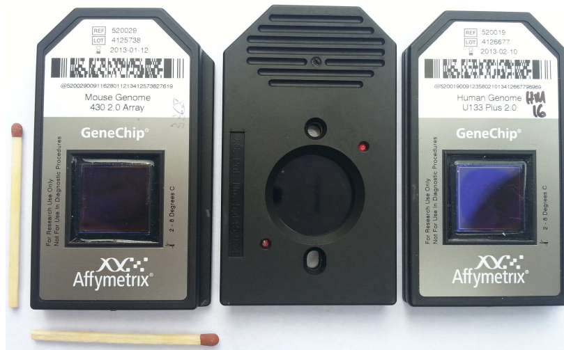
Fig. 1.2 Gene expression data are extracted from Affymetrix microarray. Two Matchsticks are placed for reference purpose. Images at the left side and right side are the top-view and middle one is the bottom view of the microarray. Left one contains mouse genome with 430 2.0 array, while right one contains human genome with U133 Plus 2.0 array. A special scanner (i.e. GeneChip scanner) is required to scan this high-density arrays.
