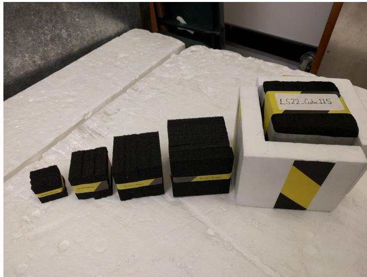
Figure 3.17: The series of absorber cuboids, made from carbon-loaded foam
