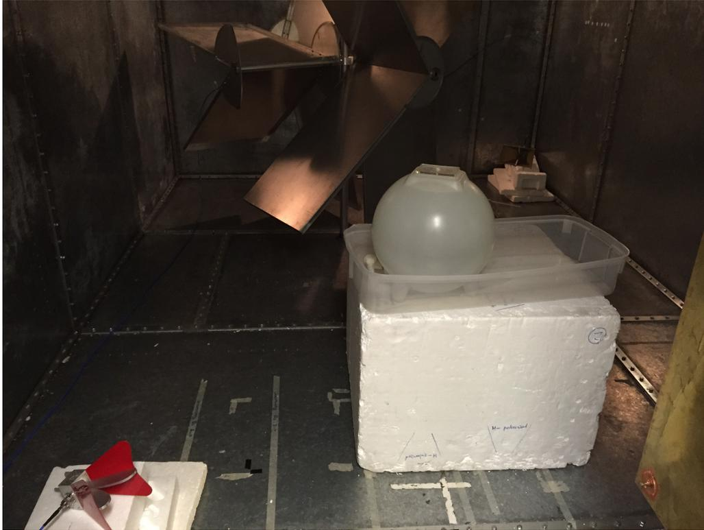
Figure 3.8: The measurement setups of the sphere model
