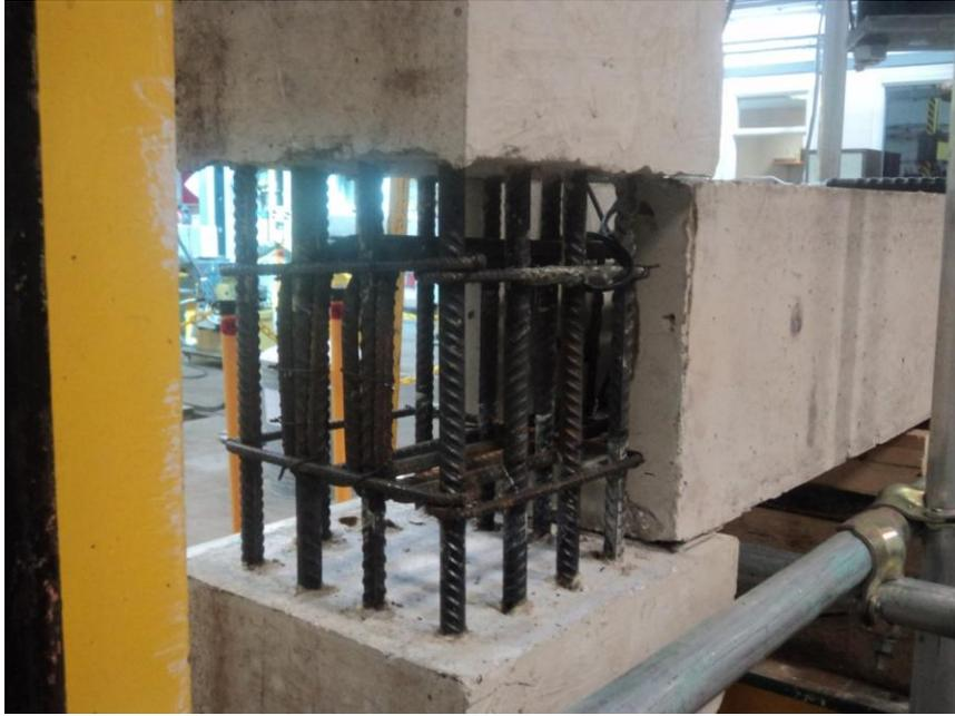
**Figure 3-11 Reinforcement detail of the joint core**
