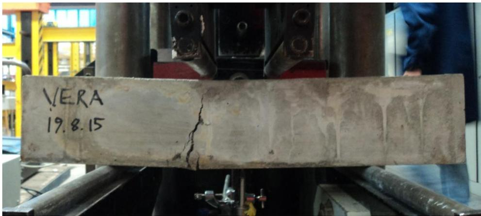
(b) Steel fibre reinforced concrete
