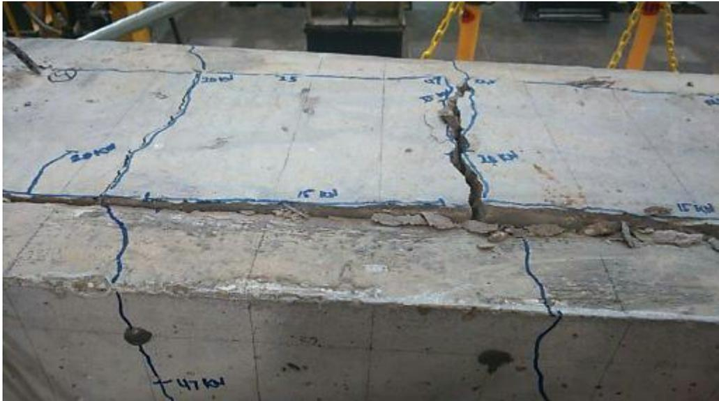
**Figure 4-23** Photo of cracks on the top surface of the beam core of Specimen P1
