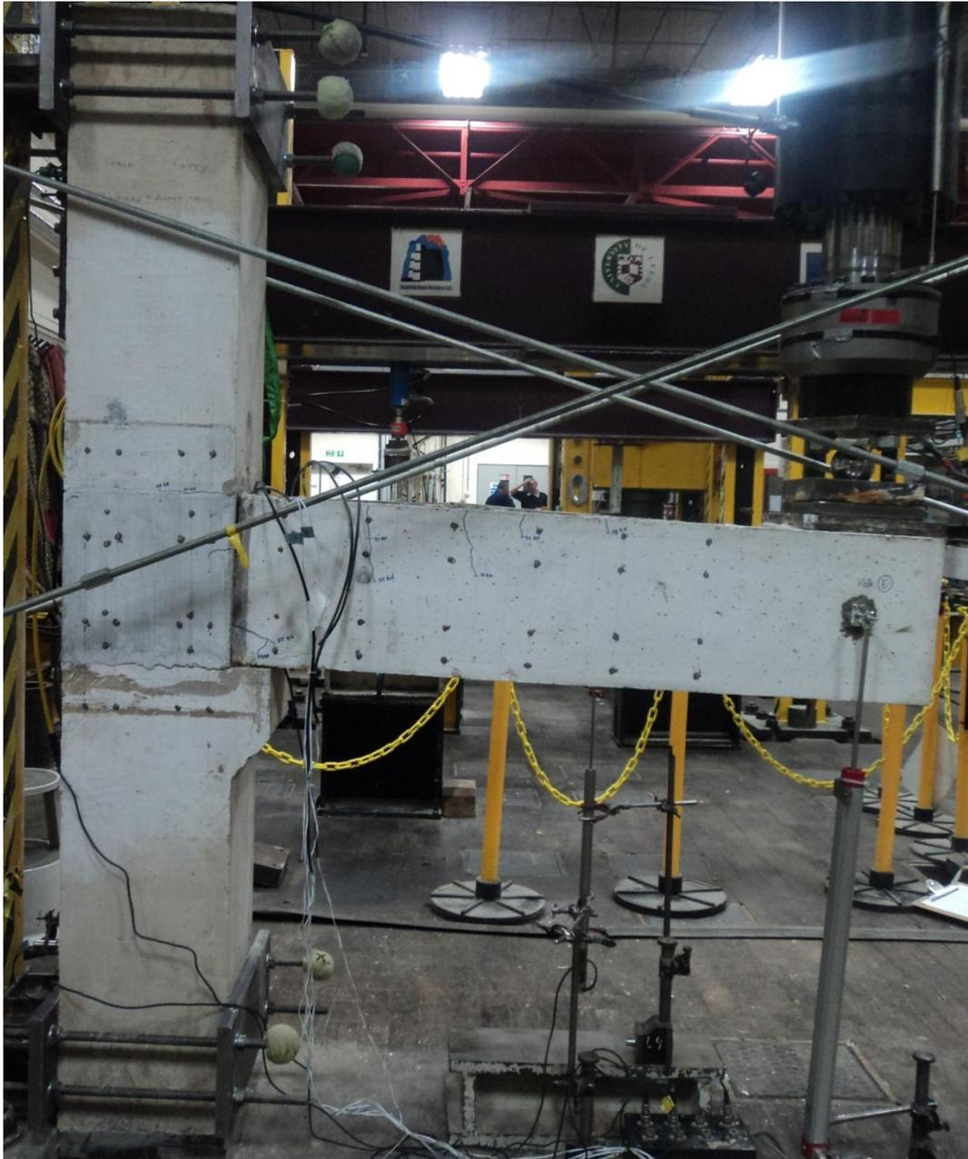
**Figure 4-6 Crack pattern of beam-column specimen subjected to static loading (Specimen P1)**
