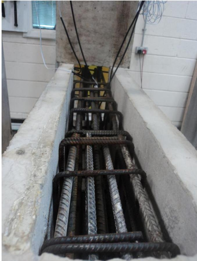
**Figure 3-12 Reinforcement detail in the CIP beam core of Specimen P1**
