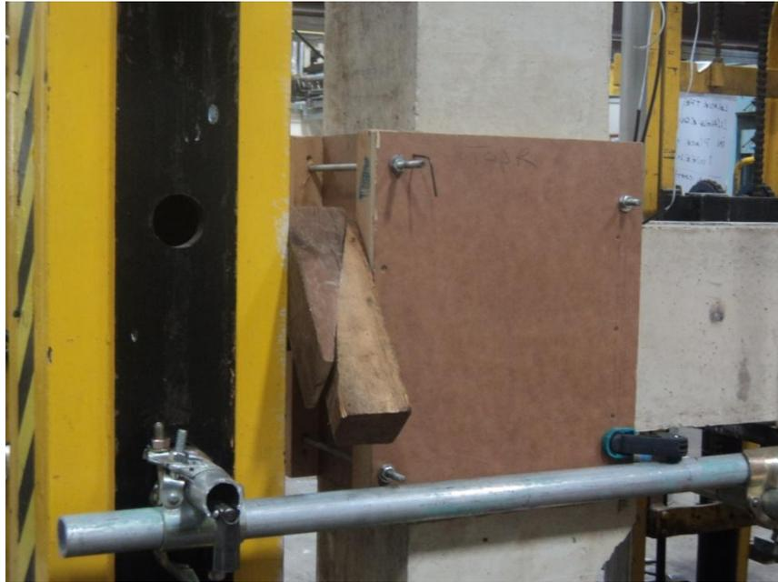
**Figure 3-14 Joint core covered by a form before casting**
