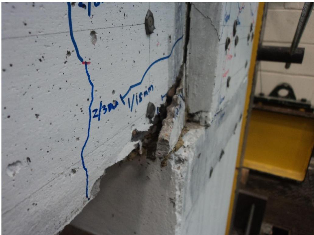
**Figure 5-10 U-beam condition Specimen P2 at the end of displacement level of 60 mm (2<sup>nd</sup> cycle)**
