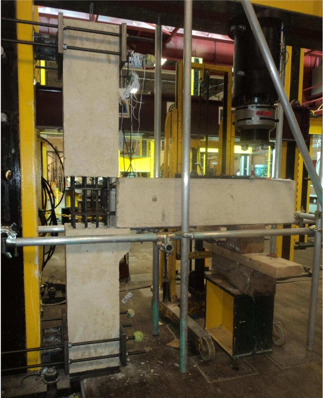
**Figure 3-10 Precast U-beam seated on the corbel of the precast column**
