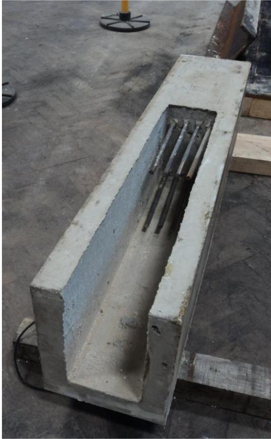
**Figure 3-8 Precast U-beam**
