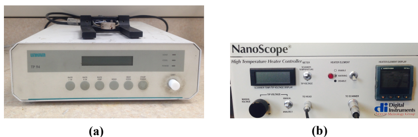
Figure 3.16: Photos of (a) the Linkam TP94 hotstage used with the Dimension AFM and (b) the Nanoscope high temperature heater controller used with the Multimode 8 AFM.
