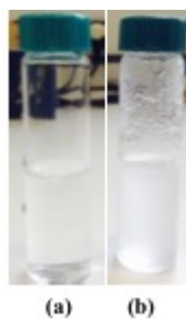
Figure 6.1: A photo of PE (a) hot solution immediately after removing it from the oil bath after dissolving the PE into the solvent at 135 °C and (b) suspension a few minutes after removing the solution from the hot bath.
