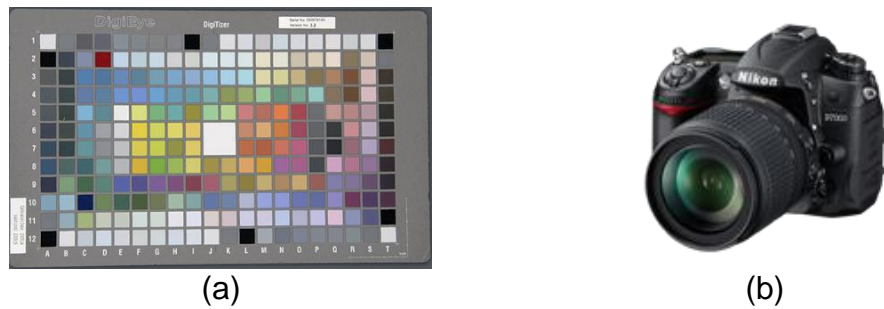
Figure 3.2.1.1 The calibration colour chart and the digital single-lens reflex camera used in the imaging system. (a) DigiTizer chart V3.3; (b) Nikon D7000.
