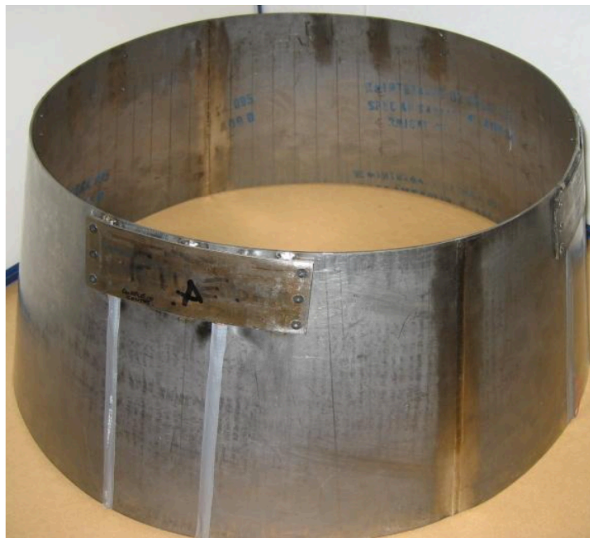
Figure 2.24: “Wavy” variable area nozzle (courtesy of ADVACT)
