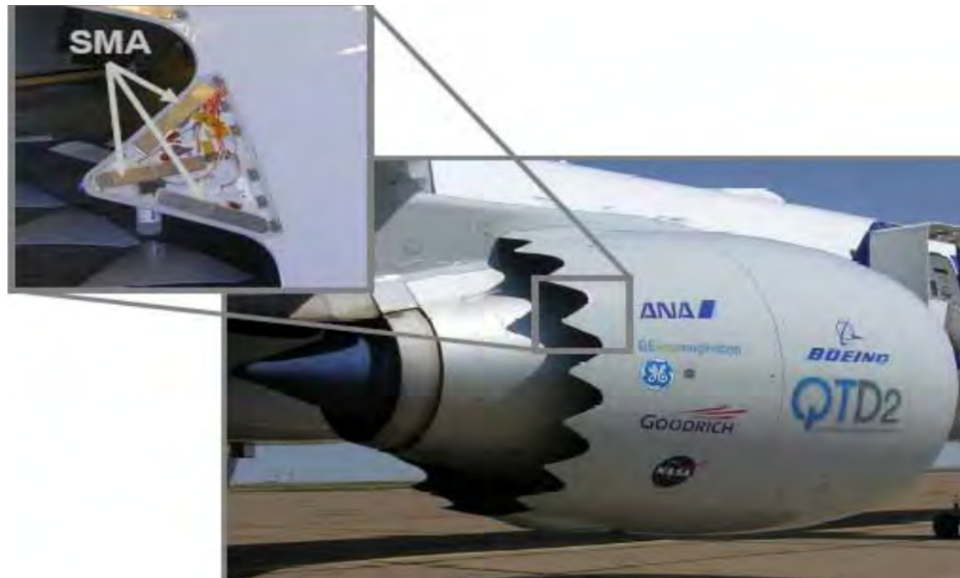
Figure 2.20: Reconfigurable engine nozzle fan chevron using SMA (courtesy of Boeing)
