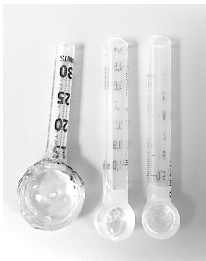
Figure 2: Customised sample holders of two sizes for imaging oviduct tissue samples. The tissue samples were pinned on the silicon elastomer surface with the UVJ mucosal surface and the SST orifices exposed.
