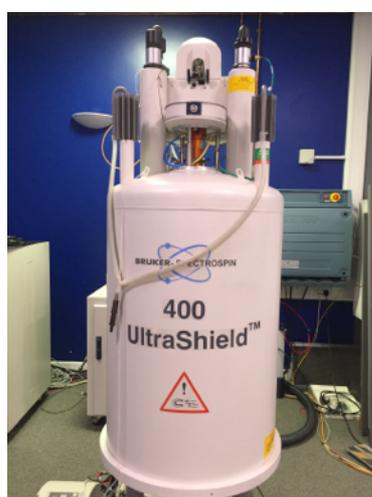
Figure 93: the vertical NMR magnet or NMR spectrometer
