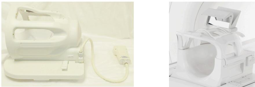
Figure 27: Image A shows the 8 channel head coil used in GE scanner and image B shows the 12 channels head coil in Siemen's scanner
