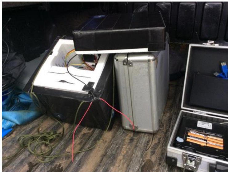
Figure 3.2. Inside the sampling box and associated GPS system.
