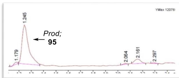
**Figure 20.** LC/MS monitoring of the photochemical formation of **95** after 140 minutes.
