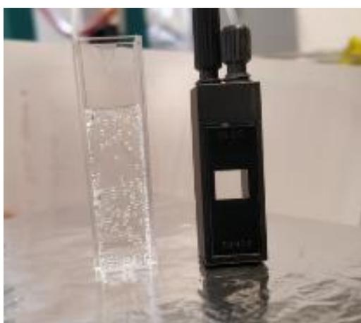
Figure 48. A plastic cuvette containing aqueous NaBH<sub>4</sub> solution (2 mM) opened to the atmosphere (left). A flow cell containing aqueous NaBH<sub>4</sub> solution (2 mM) under 40 psi of pressure showing the formation of H<sub>2</sub> gas bubbles in a non-pressurised cuvette.
