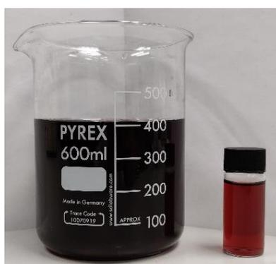
Figure 86. An image showing 400 mL of AuNPs collected from the fReactor CSTR.
