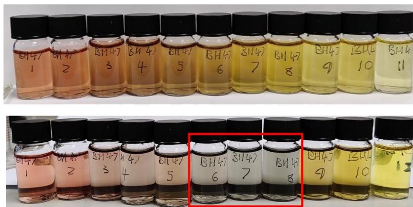
Figure 77. A photograph showing the nanoparticle solutions produced immediately after flow synthesis (Top) and one hour after synthesis (bottom), with black precipitate highlighted in the red box.
