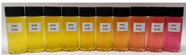
Figure 60. Sample vials containing a range of AuAgNPs with increasing gold concentrations from left to right.
