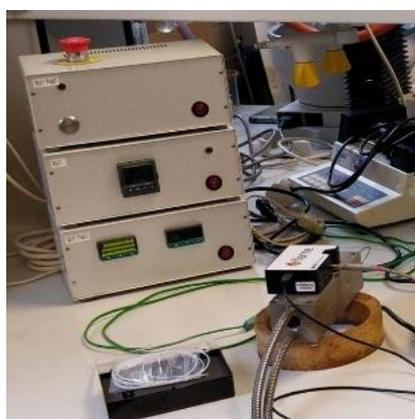
*Figure 49. UV-vis spectrometer placed on top of an aluminium heating block regulated with a Eurotherm PID controller.*
