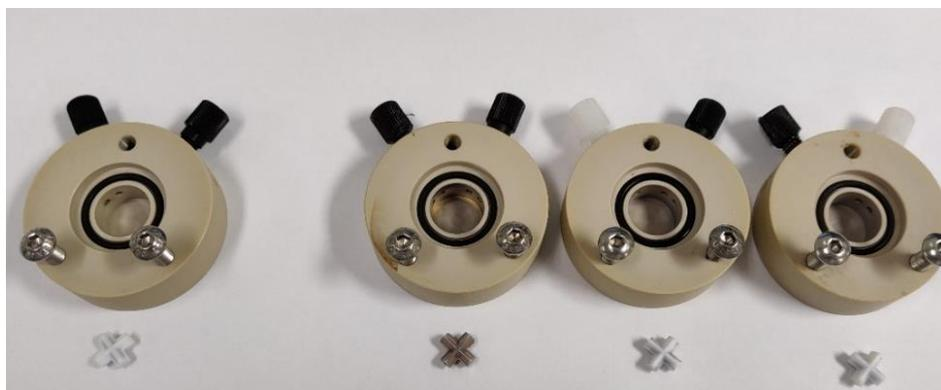
Figure 90. Clean fReactor (left) followed by stages 1, 2 and 3 (right), fouling was observed only within the first reactor of the series.
