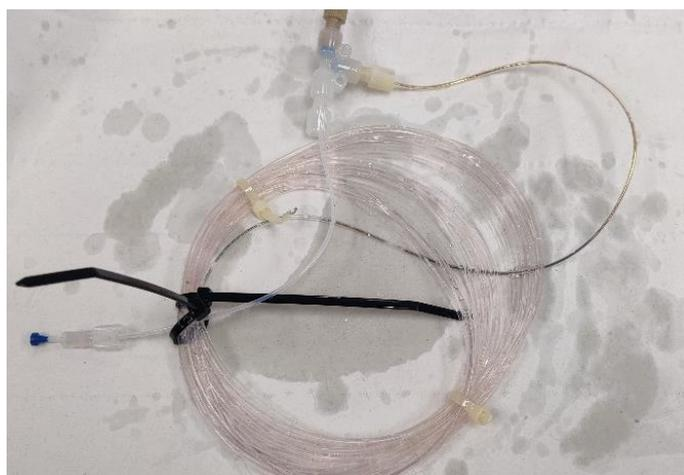
Figure 80. An image showing the PFA reactor tubing after approximately 1 hour of use, the internal wall of the first 30 cm of the reactor tubing is coated in metallic gold.
