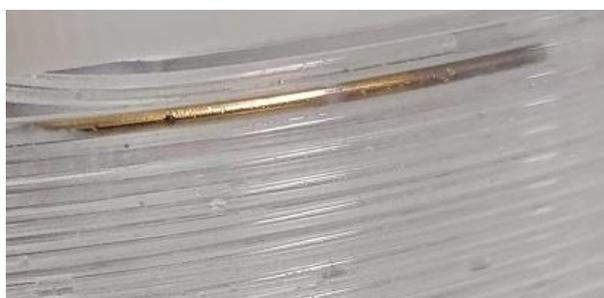
Figure 66. An image showing gold nanoparticles accumulating to form solid gold on the reactor walls.
