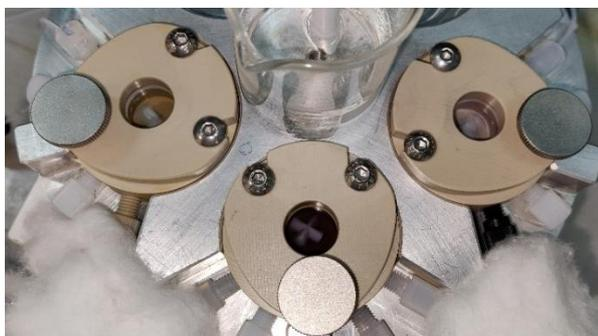
Figure 83. A photograph showing the fReactors used to synthesise AuNPs, cotton wool was used to insulate the tubing connections between the preheating fReactors and the main fReactor.
