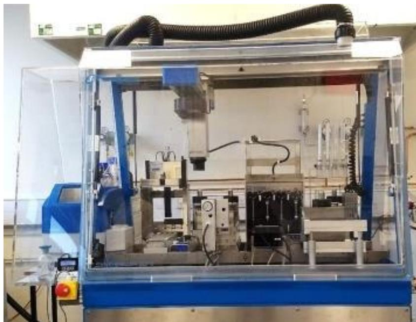
*Figure 123. A photograph of a ChemSpeed catalyst screening platform used to screen catalysts and reaction conditions in an automated fashion (Photo credit: Christopher Horbaczewskij, University of York, 2021).*
