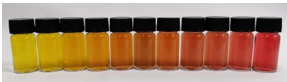
Figure 92. A photograph of the AuAgNPs showing the effect of alloy composition on the colour of the nanoparticle solutions, with the samples from left to right increasing in Au composition. Far left 100% silver with samples increasing in gold content by 10% up to 100% gold on the far right.
