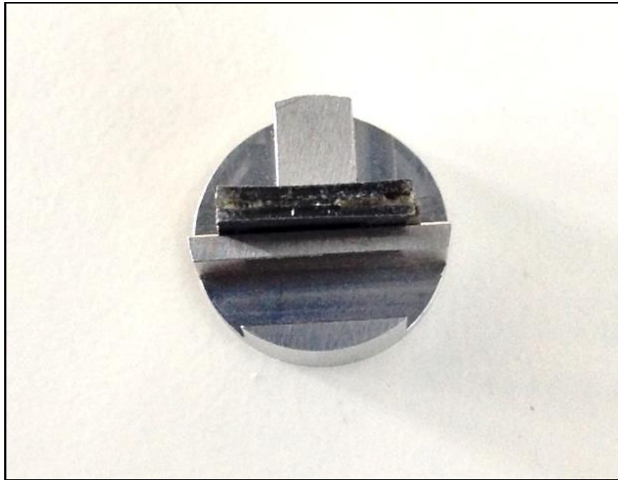
Figure 4.2. : The cryogenically fractured surface employed for investigating the nano-mechanical properties.
