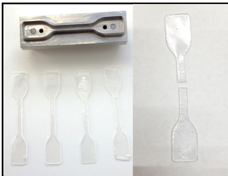
Figure 3.5.: The dumbbell, samples taken from the nanocomposites' films by the dumbbell, and the region of fracture for a tested sample
