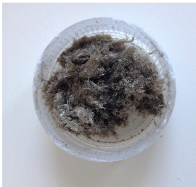
Figure 3.3. : The fluffy powdered material of GO obtained by freeze drying.
