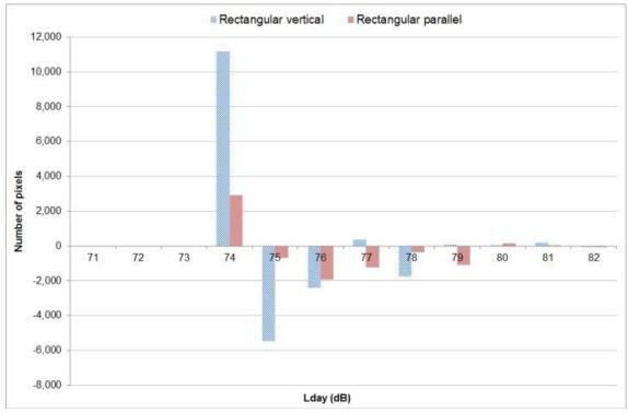
**Fig.3.9**. Comparison between the vertical and parallel to the inner road green space arrangement for the rectangular configuration as shown in Fig.3.7. The total number of pixels per noise band on the y axis is calculated by subtracting the ones in the rigid condition (G=1) from the ones in the porous condition (G=0).
