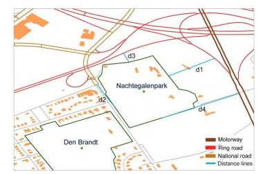
**Fig.6.4.** Example of the road categories around the Nachtegalenpark and the calculated distances from the centre of each side (*d1*, *d2*, *d3*, *d4*).
