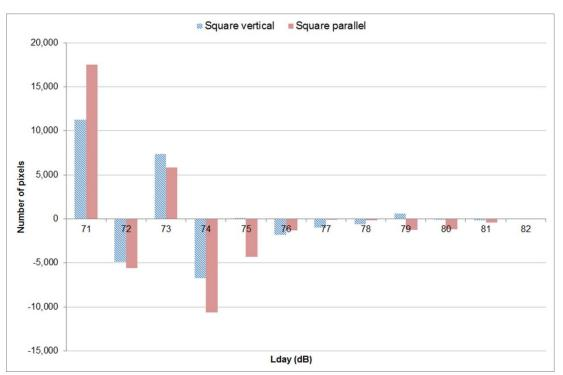
**Fig.3.8.** Comparison between the vertical and parallel to the inner roads green space arrangement for the square configuration as shown in Fig.3.6. The total number of pixels per noise band on the y axis is calculated by subtracting the ones in the rigid condition (G=1) from the ones in the porous condition (G=0).
