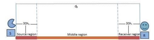
Fig.3.2. Example of source (s) and receiver (r) region in ground attenuation according to ISO 9613-2.
