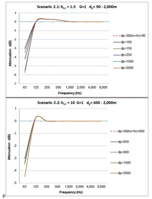
Fig.3.4. Scenario 2: Ground attenuation per octave band for G=1, dp=1.5-2,000m and (a) hs,r =1.5m, (b) hs,r =10m
