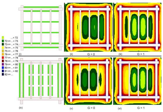
Fig.3.6. Noise propagation in a square form tested with different ground factors and green lanes placed in a vertical (ii,iii) and parallel arrangement (v, vi) to the inner roads.
