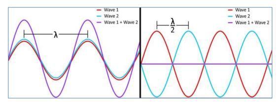
Fig.2.1. Example of positive interference (left) and negative (right) with the subsequent changes in the wave length. Source: http://angstromengineering.com/thin-film-u/introduction-optical-coatings/
