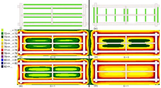
Fig.3.7. Noise propagation in a rectangular form tested with different ground factors and green lanes placed in a vertical (ii,iii) and parallel (v,vi) arrangement to the inner road.
