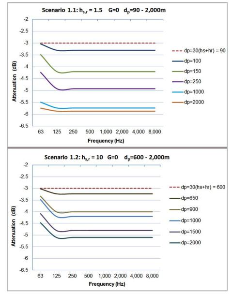
Fig.3.3. Scenario 1: Ground attenuation per octave band for G=0,  $d_p$ =1.5-2,000m and (a)  $h_{s,r}$ =1.5m, (b)  $h_{s,r}$ =10m
