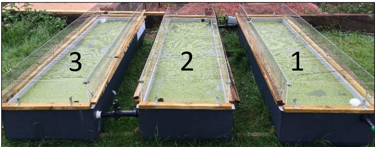
Figure 5.2.1.5. Duckweed tank layout. WW entered tank 1 inlet (bottom right corner) and continued through tanks 2 and 3 via ventilated sub-surface connections where gravity returned WW back to discharge tank. Clear Perspex screens were installed for wind protection and netting to prevent wildlife (birds/small mammals) from invading.
