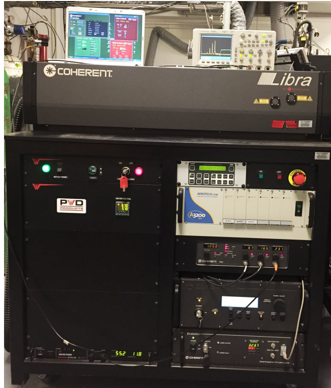
Figure 2.2: Libra ultra fast laser amplifier system
