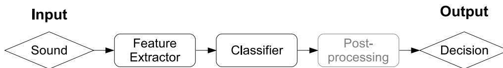
Figure 1.1: Flow diagram showing the basic structure of a classification system. Adapted from Allegro, Büchler, and Lawner (2001).
