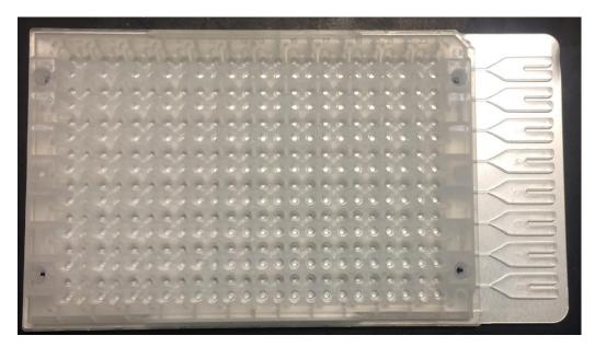
**Figure 2.6. TLDA microfluidic card.** Each card contains 8 ports that will supply the 384 wells with the PCR reaction mix.
