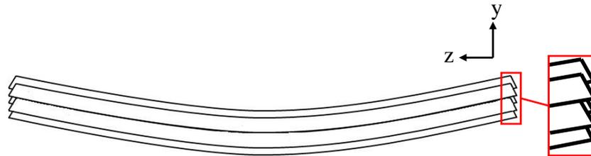
Figure 6.2 Typical multi-strand bar undergoing flexure (seven-strand bar shown)
