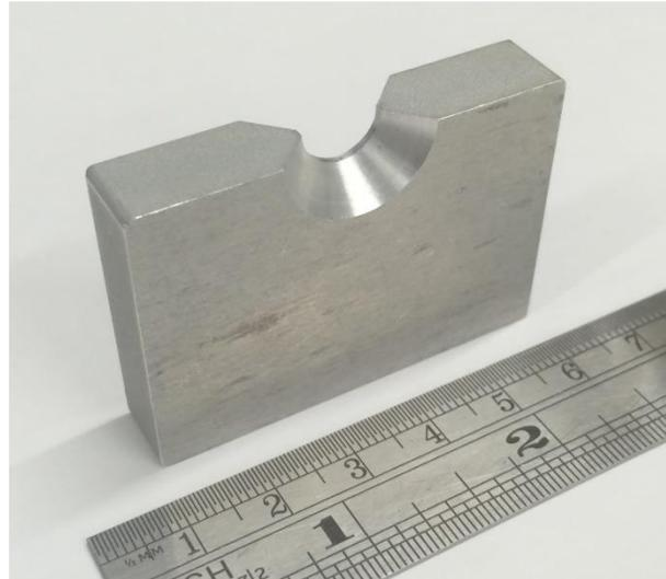
Figure 6.24 Support bearing
