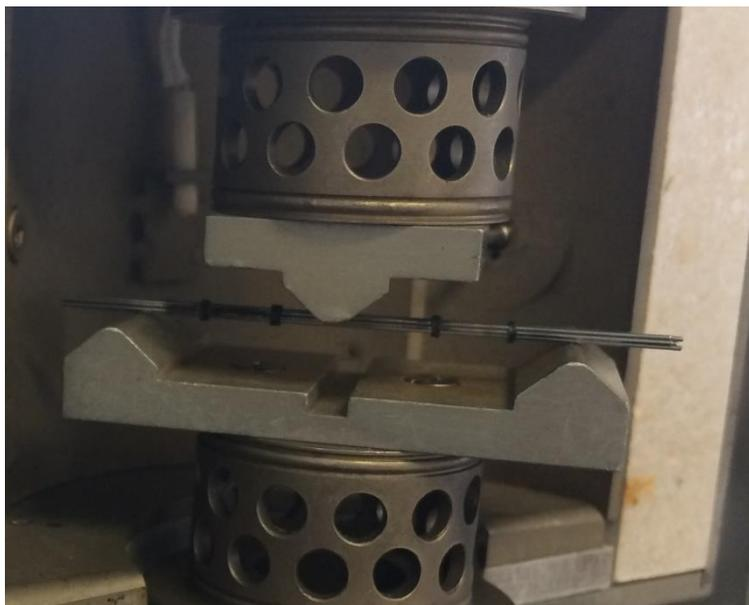
Figure 6.32 Seven-strand wire during the three point flexure loading
